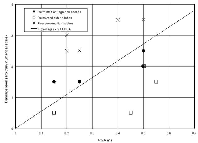
FIGURE 2 Northridge earthquake damage versus peak ground acceleration (PGA) for adobes other than unreinforced and well-maintained.
