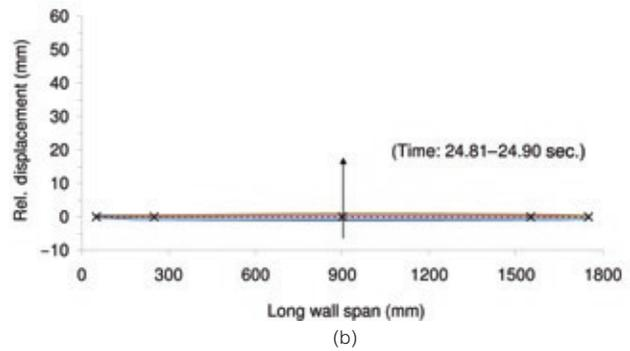
FIGURES 9A AND 9B Specimens 3A and 3F during simulation S6 (75%): horizontal flexure of top of long wall for specimen 3A (a) and specimen 3F (b).
