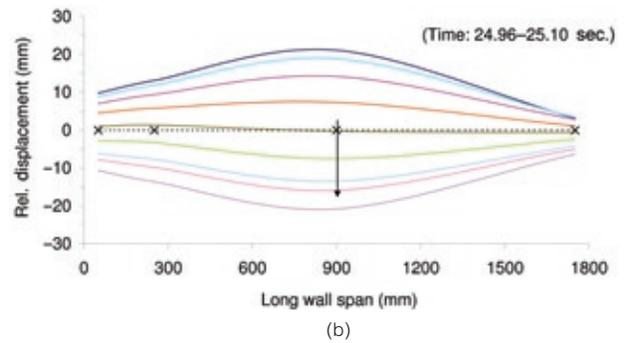
FIGURES 10A AND 10B Specimens 3F and 3K during simulation S8 (125%): horizontal flexure of top of long wall for specimen 3F (a) and specimen 3K (b).
