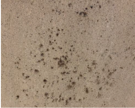
Image 1. Black fungus-like surface deposit on outdoor Cemesto panel. Sample 4.
