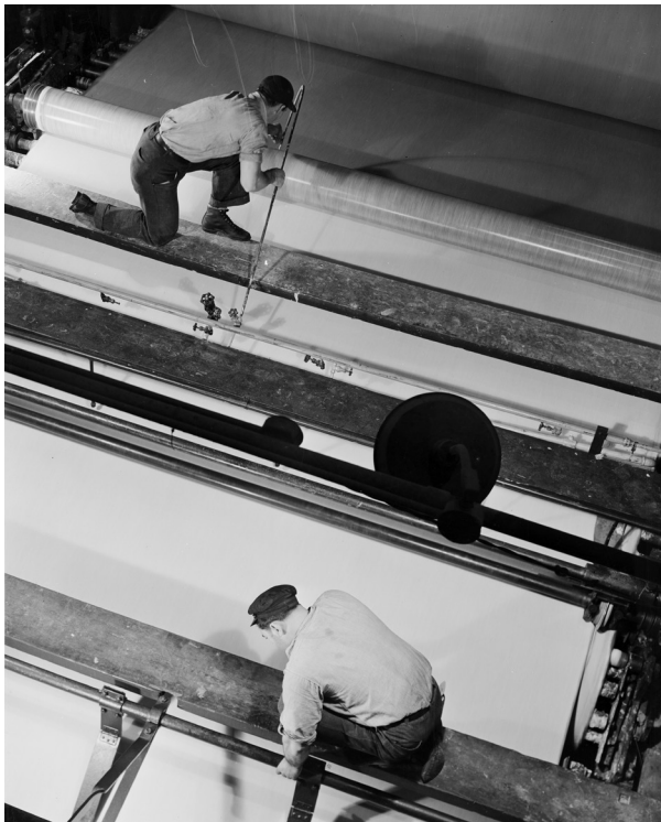
FIGURE 1.5 Workers passing the fiber mixture through rollers that felt the fibers together, squeezing the water out and causing the fibers to adhere into a continuous sheet. Photo: Robert Yarnall Richie, Celotex, Marrero, Louisiana (12/38) for Fortune magazine. Robert Yarnall Richie Photograph Collection. Ag1982.0234. DeGolyer Library, Southern Methodist University.
