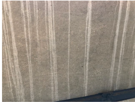
Image 2. White stripes on surface of indoor Cemesto panel (HE-35). Sample 1.
