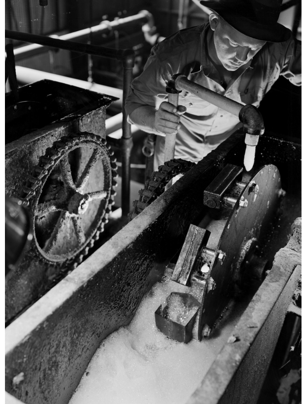
FIGURE 1.4 The cooked and cleaned fiber mixture in the process of being shredded to a soupy consistency using mechanized rotating hammers. Photo: Robert Yarnall Richie, Celotex, Marrero, Louisiana (12/38) for Fortune magazine. Robert Yarnall Richie Photograph Collection. Ag1982.0234. DeGolyer Library, Southern Methodist University.
