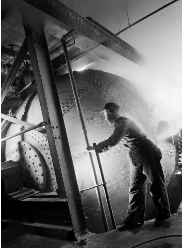
FIGURE 1.3 A worker operating equipment in which the bagasse is heated, or cooked, to soften the fibers. Photo: Robert Yarnall Richie, Celotex, Marrero, Louisiana (12/38) for Fortune magazine. Robert Yarnall Richie Photograph Collection. Ag1982.0234. DeGolyer Library, Southern Methodist University.
