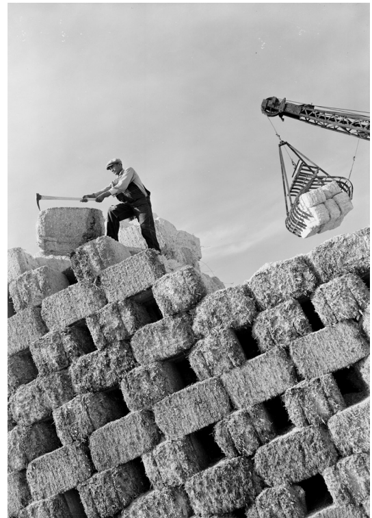
FIGURE 1.2 Photo showing bales of bagasse drying prior to delivery to the manufacturing plant. Photo: Robert Yarnall Richie, Celotex, Marrero, Louisiana (12/38) for Fortune magazine. Robert Yarnall Richie Photograph Collection. Ag1982.0234. DeGolyer Library, Southern Methodist University.
