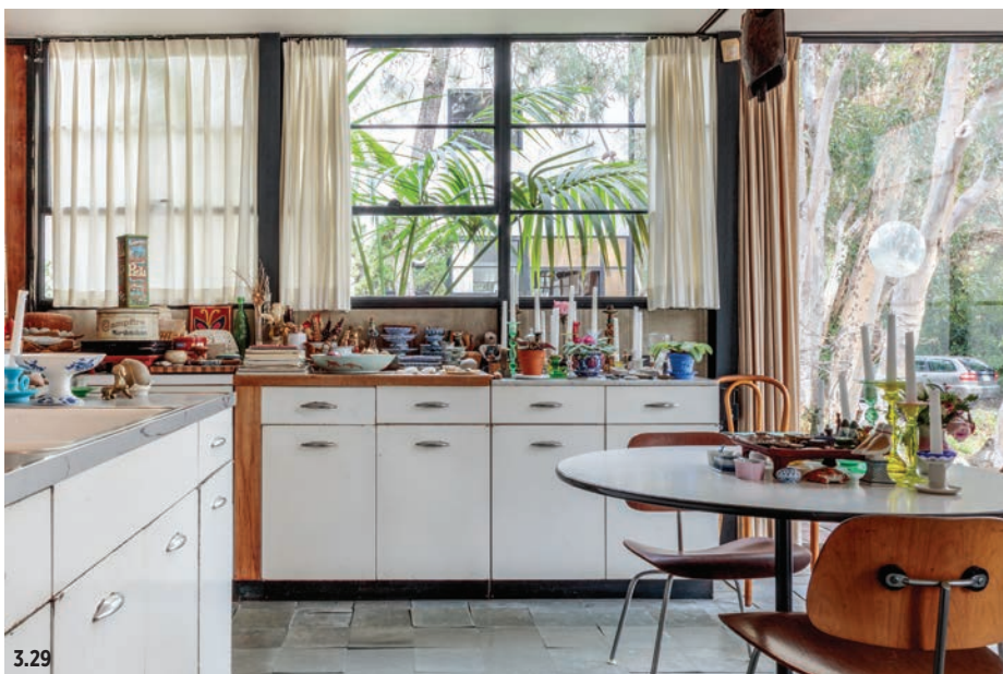
Figure 3.29 North wall of the kitchen in 2017, showing the prefabricated steel cabinets and window units filled with clear glass and hung with curtains. At right, the steel-framed sliding door opens to the central court.
