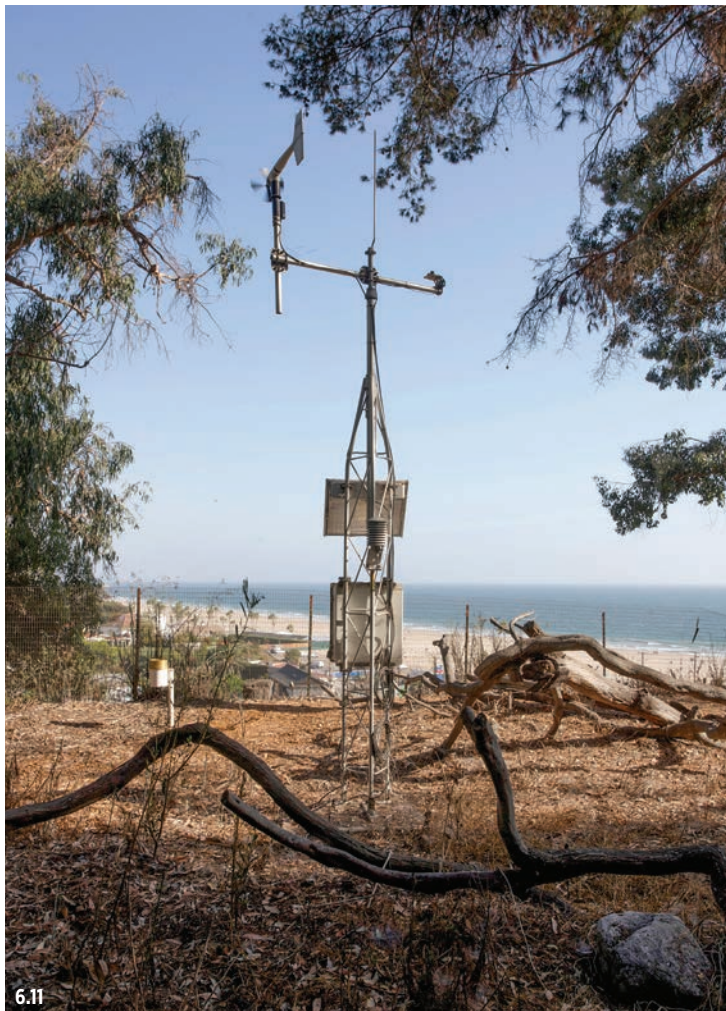
Figure 6.11 Weather station installed by the GCI in the meadow, 2016. Environmental monitoring began in 2011 to gather baseline temperature, humidity, and wind data that will inform environmental improvement recommendations.
