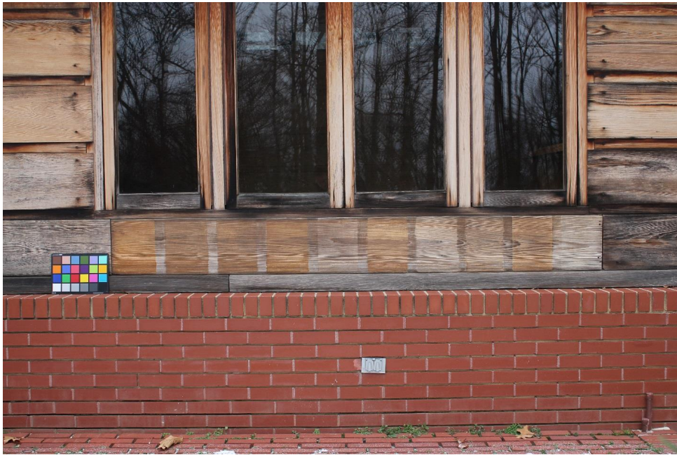
FIGURE CS-C.7 Field testing of TWP products on cypress since 2011 at Frank Lloyd Wright's Pope Leighey House, Alexandria VA. January, 2013. Photo: Courtesy of Frank Lloyd Wright's Pope-Leighey Project, Andrew Fearon, Pamela Kirschner and Ashley Wilson
