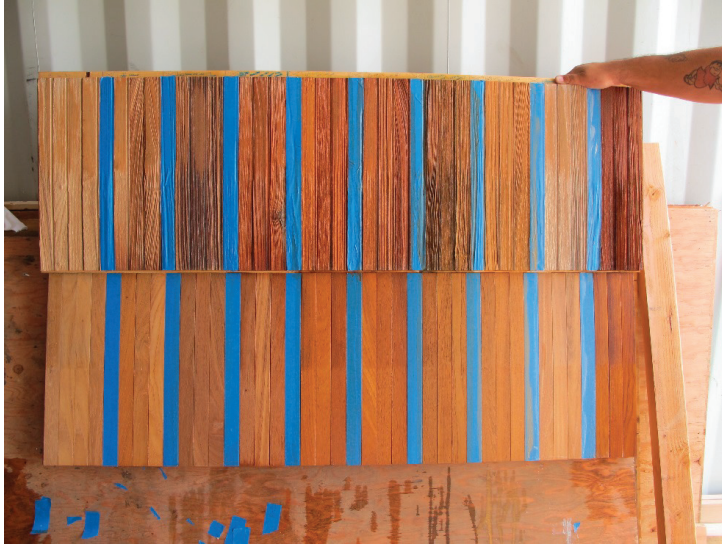
FIGURE CS-B.13 View of Mock-Up 4, trialing finishes on existing weathered teak (top panel) and new FEQ teak (lower panel), May 4, 2015. Treatments trialed (from left to right) are untreated, Wolman Woodlife Classic Clear Wood Preservative, Sansin Wood Sealer (2 coats), Nissus Boracare with Sansin Wood Sealer, Gemini Coatings TWP 400 Series Light Cedar 415, Gemini Coatings TWP 1500 Series Pecan 1520, Sansin SDF Natural Suede 19, Sansin SDF Transluents Custom Tinted, Benjamin Moore Arborcoat waterborne exterior stain translucent silver grey 623-70, and Messner's UV Plus for Hardwoods Natural. These panels will be placed on the roof of the Salk Institute at southwest exposure to observe the weathering processes. Photo: J. Paul Getty Trust
