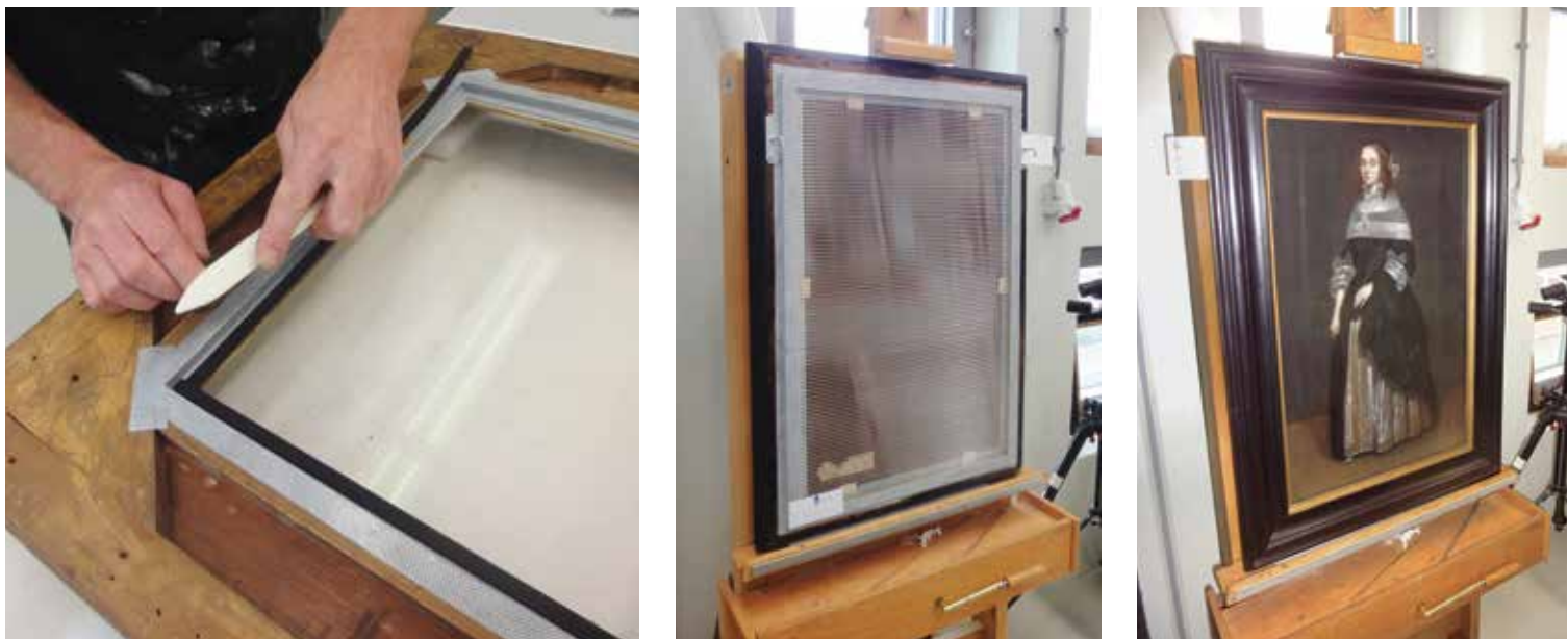
Figure 4. Constructing a microclimate frame: sealing glass in frame; attaching airtight backboard; invisible from the front. Photos: Bart Ankersmit/RCE.
