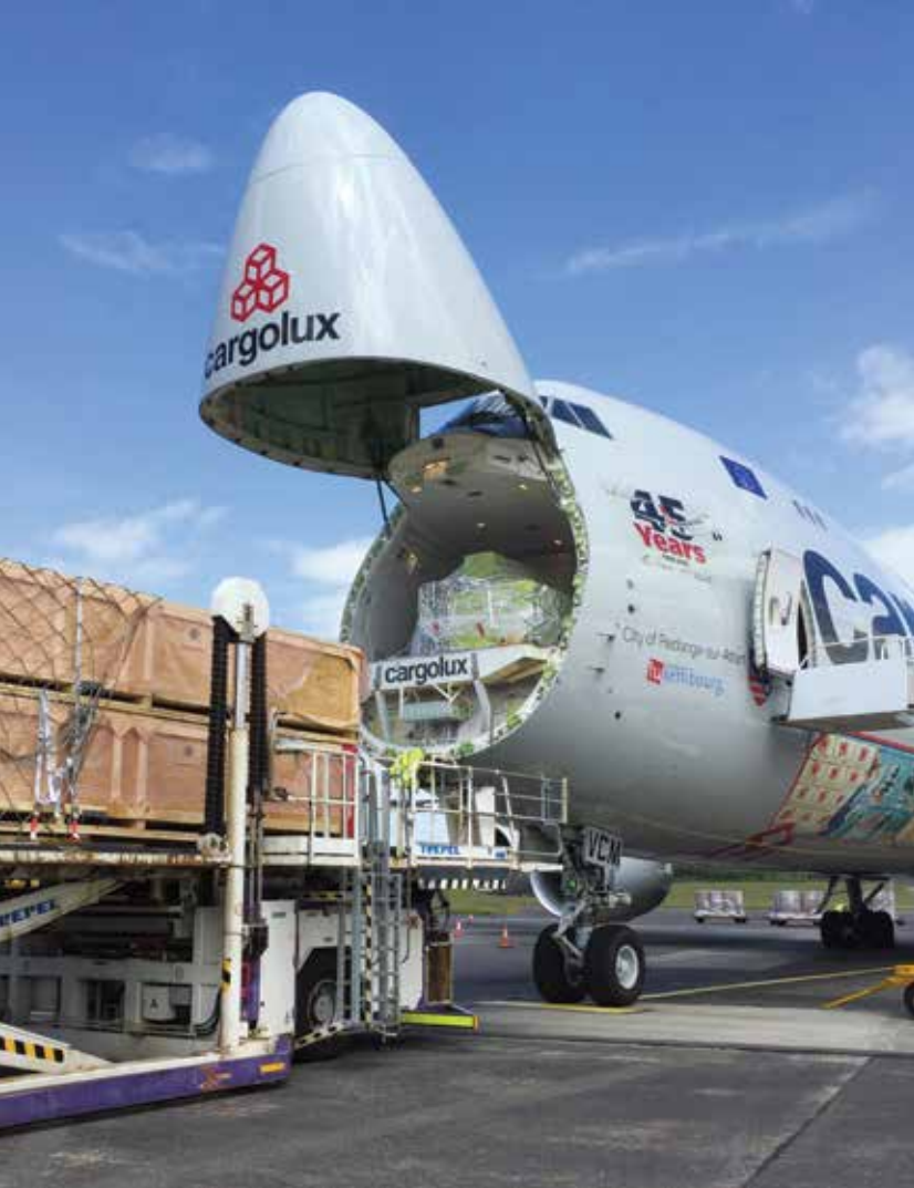
A pallet of crates loaded into the nose cargo door of a Boeing 747-8F purpose-built freight aircraft. The nose door allows for cargo that might be too large or long to fit through the side cargo door. It also facilitates easier access to front-loaded pallets on transit flights. Photo: Judy Chiba Smith, courtesy of the Georgia O'Keeffe Museum.
