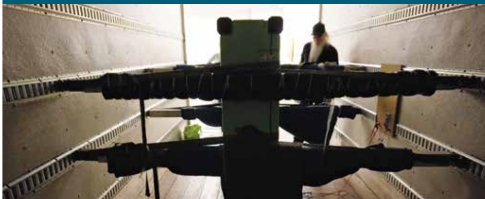
Kevin Marshall, former head of preparations at the Getty Museum, using crossbars to secure a crate in a box truck. Photo: Gina Eichmüller.
