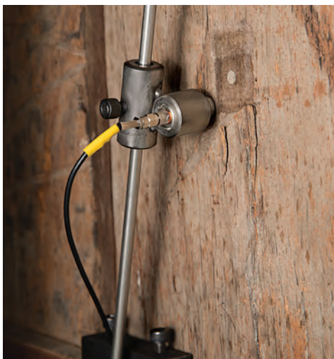
Custom-designed mounting system for an acoustic emission sensor on the 16th-century retablo in the National Gallery of Victoria, Melbourne. Photo: Predrag Čančar, National Gallery of Victoria.
