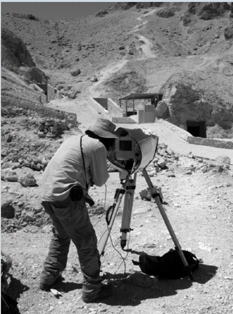
A member of the survey team conducting laser scanning at the Valley of the Queens in Egypt. This work will be used to generate an accurate, GIS-based topographic map indicating the locations of tombs, other ancient features, and modern infrastructure. Photo: David Myers.
