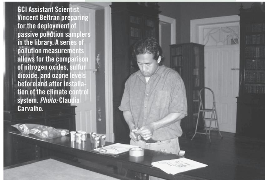
GCI Assistant Scientist Vincent Beltran preparing for the deployment of passive pollution samplers in the library. A series of pollution measurements allows for the comparison of nitrogen oxides, sulfur dioxide, and ozone levels before and after installation of the climate control system. Photo: Claudia Carvalho.
