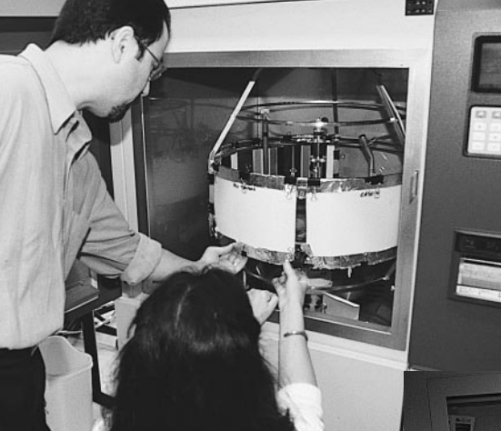
Left: GCI project team members Herant Khanjian and Valerie Dorge installing the prepared paint films in the Atlas Weather-Ometer in the GCI scientific laboratories. The films were subjected to 12 weeks of artificial aging, simulating a museum environment. Photo: Dusan Stulik.
