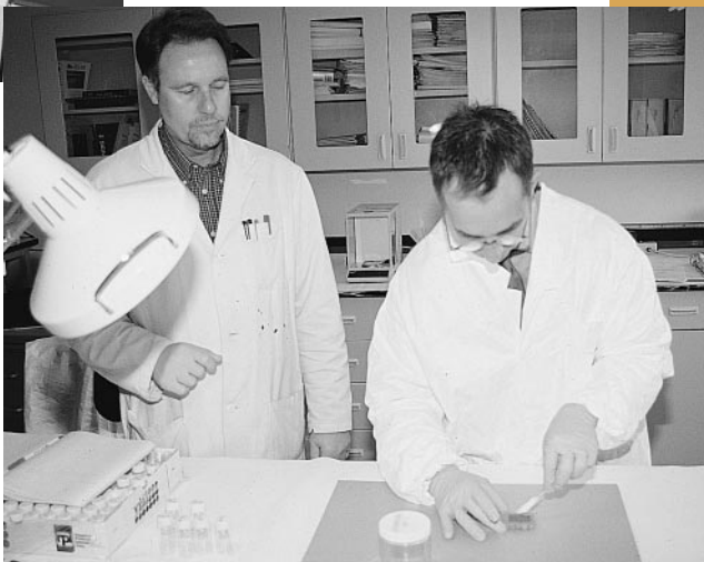
Right: Brian Considine (right), Getty Museum decorative arts conservator, and David Miller (left), professor of chemistry at California State University, Northridge (CSUN), conducting a cleaning experiment on a gilded wood sample in the CSUN chemistry laboratory. The objective of the experiment is to determine the amount of residue left on the gilded surface after the gels cleaning process. Photo: Valerie Dorge.
