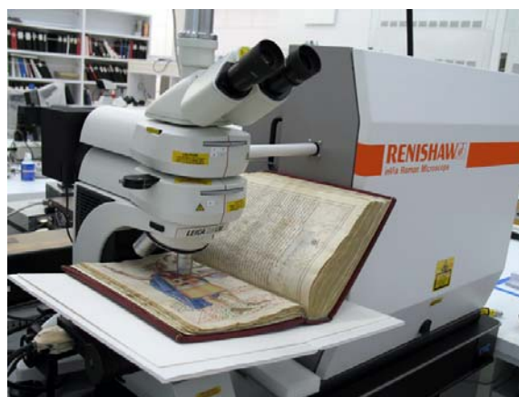
Getty Murúa being examined using the GCI's Renishaw Raman spectrometer.
