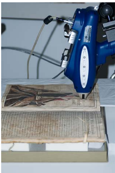
Galvin Murúa being examined using the GCI's Bruker portable XRF spectrometer.
