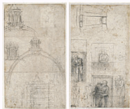
14. Michelangelo Buonarroti Italian, 1475 - 1564 Section through the Dome of Saint Peter's Basilica with Alternative Designs for the Lantern; Figure Sketches (recto); Ground Plan Showing the Base of the Lantern of Saint Peter's Basilica with Volutes; Figure Studies (verso) , 1547-61 Black chalk, leadpoint, and stylus (recto); black chalk and stylus (verso) Unframed: 39.9 × 23.5 cm (15 11/16 × 9 1/4 in.) Teylers Museum, Haarlem, purchased in 1790 Images © Teylers Museum, Haarlem EX.2020.1.12
