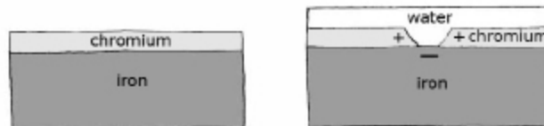
cathodic protection - chromium plating on iron
