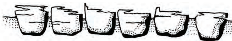
Delamination of tesserae
