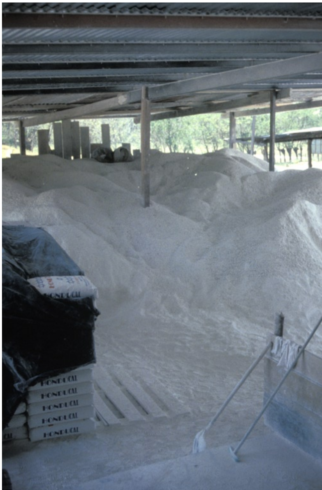
Figure 97 Powdered lime hydrate ready for bagging (foreground) and discarded, unburnt lime (background), Chiquilas, Honduras.
