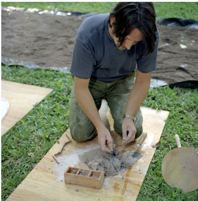
Figure 99 Preparation of the trial mortars for laboratory testing.
