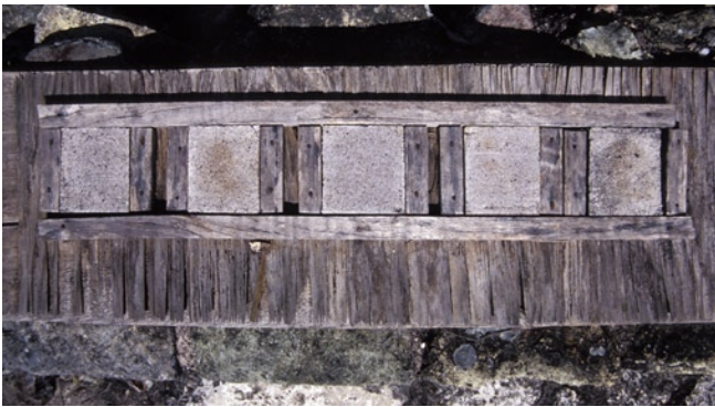
Figure 102 Lime-based mortar trial samples made in December 2001, shown after three years of unsheltered exposure at the top of the Stairway. December 2004.
