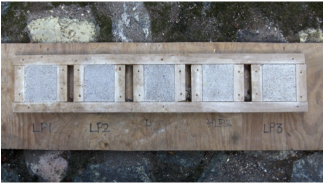
Figure 101 Lime-based mortar trial samples made in December 2001, shown after two and a half years of sheltered exposure on the Stairway. August 2004.
