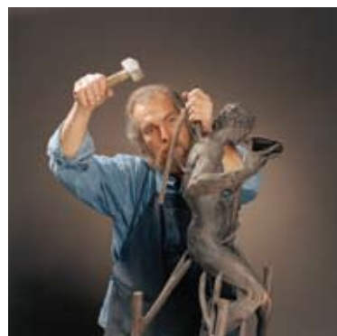
12. Chiseling a sprue off of the cast bronze.
