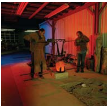
11. Crucible moved with tongs to pouring ring.
