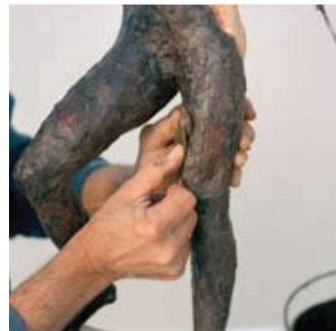
4. Modeling the wax over the clay core.
