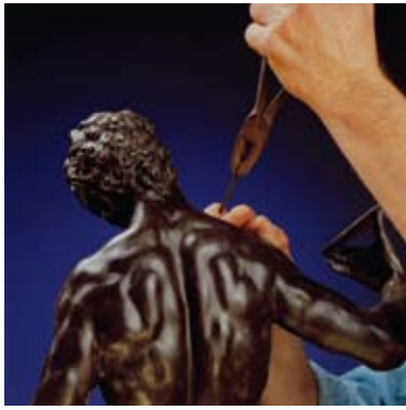
7. Putting iron core pins into the model.
