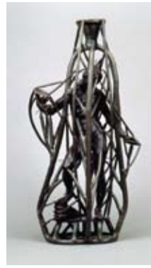
8. Model with wax pouring cup and sprues added. The sprues create channels that will allow bronze to flow into the mold and allow air and gasses out.
