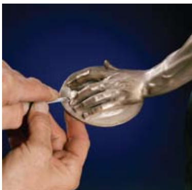
13. Sharpening surface details with a graver.
