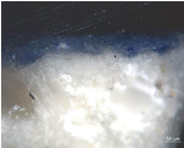
19-051-2b Microphotograph of the paint cross section under incident polarized light
