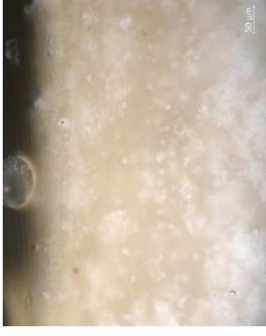
19-051-10 microphotograph of the paint cross section under incident polarized light : minimal yellow pigments
