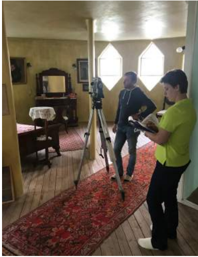
High-precision measurements of inter-floor deflections
