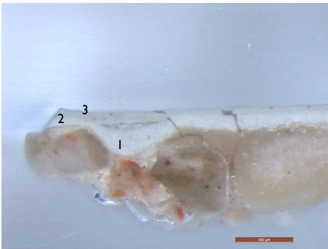
Sample 144. Dining room wall by the window. Scale 500µm. Sample broke in two parts, below are the undermost layers.
