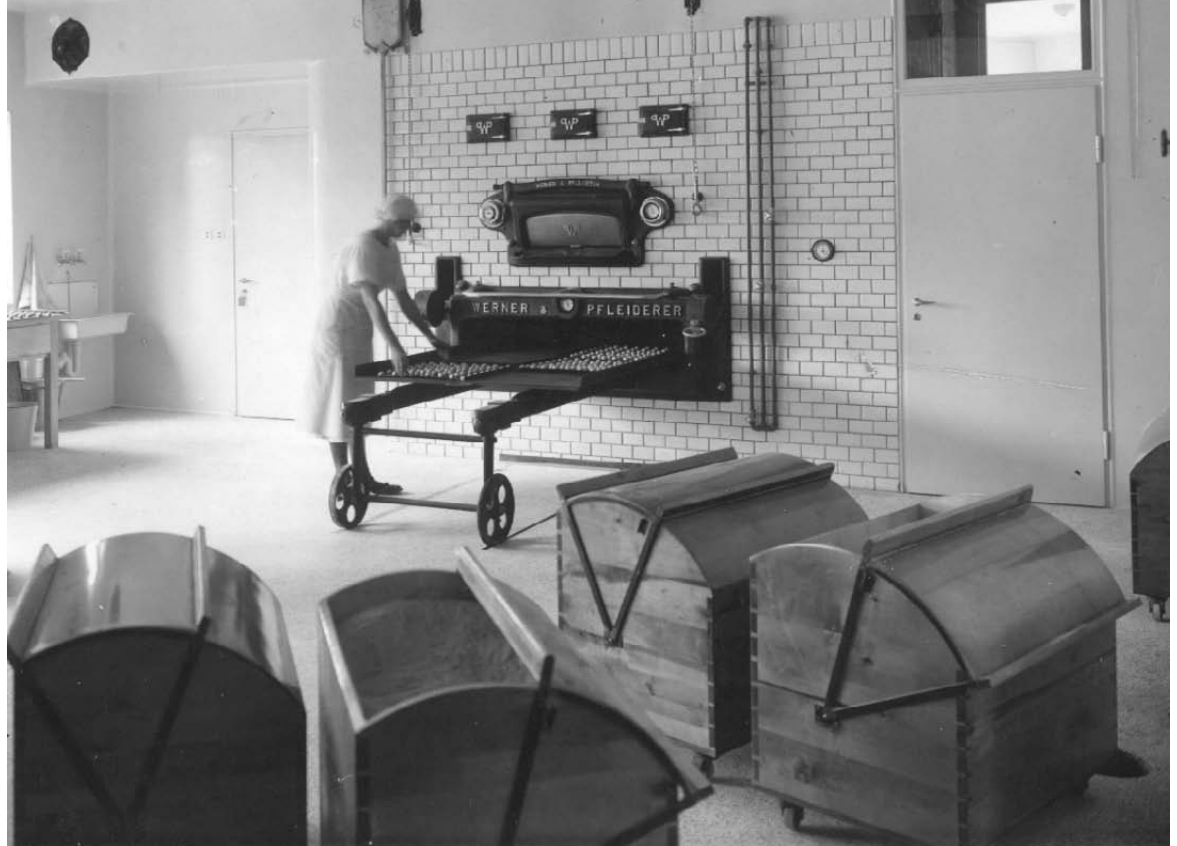
The baking oven on the basement level, an air outlet fan is visible in the far left corner (AAM 50-003-393 Gustaf Welin 1933).
