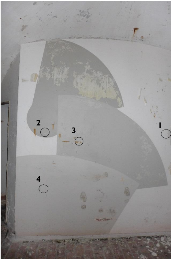
The cross section samples taken from the mural of Rose cellar.
