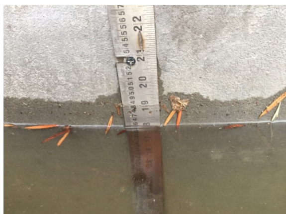
Figure 96 Monitoring of water level after treatment and loss of water recorded for 2 weeks
