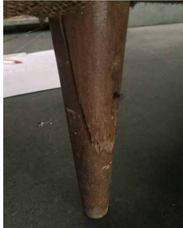
CRACK IN LEFT FRONT LEG
