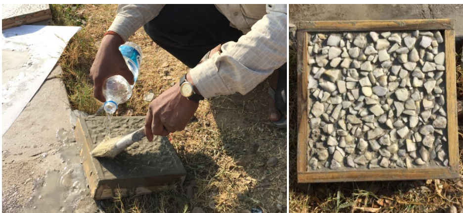
Figure 106 Top layer Cleaning of sample with water & soft brush and Wet sample
