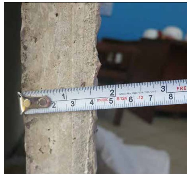
40 MM THICK GRIT PANEL WITH TOP LAYER OF EXPOSED GRIT 5MM AND BOTTOM LAYER OF CONCRETE BASE 35 MM
