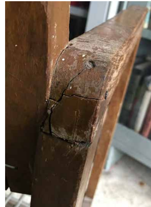
CRACKS IN RIGHT ARM REST
