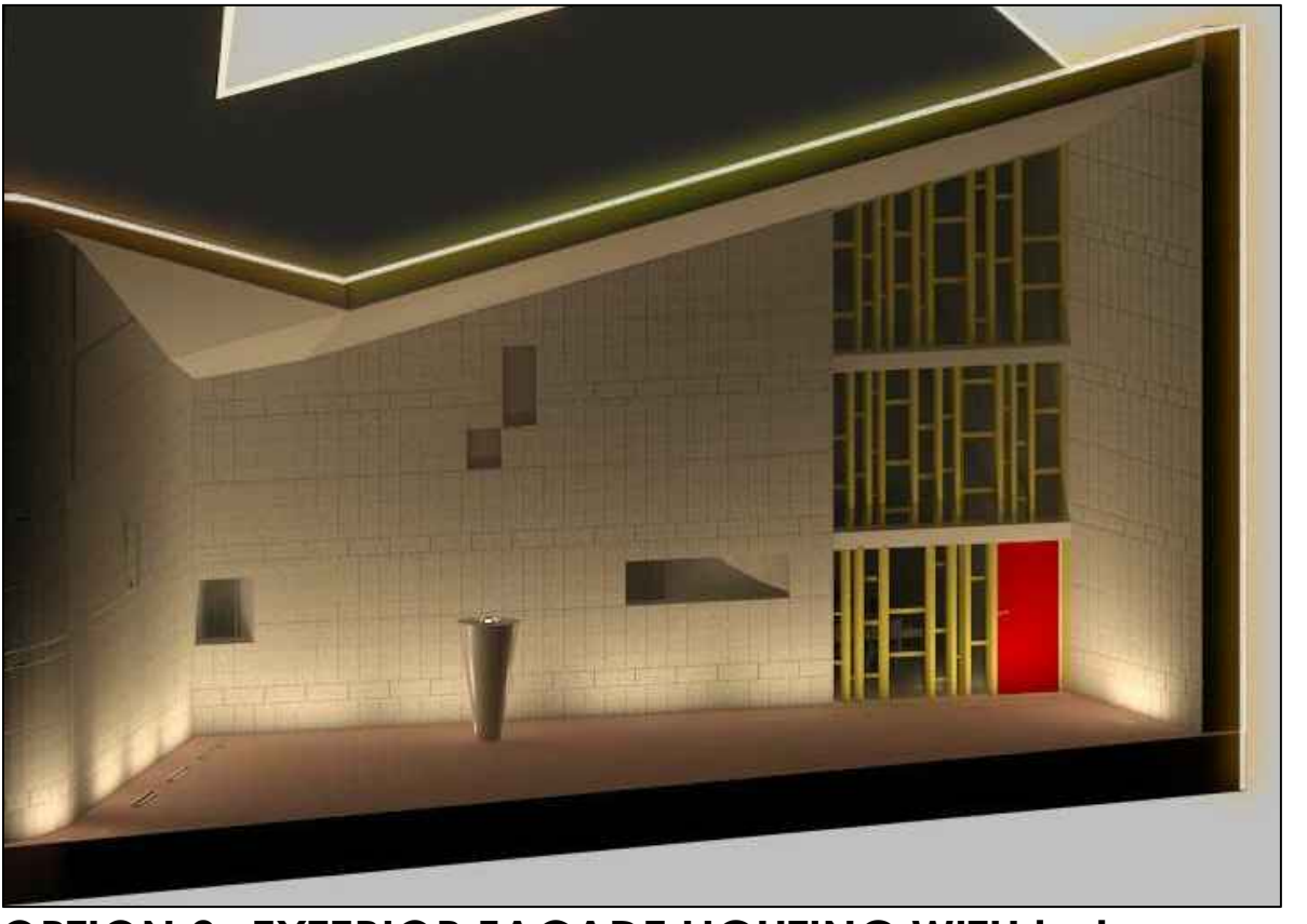
OPTION 2- EXTERIOR FACADE LIGHTING WITH led STRIP LIGHTING ON ROOF TO HIGHLIGHT THE FORM
