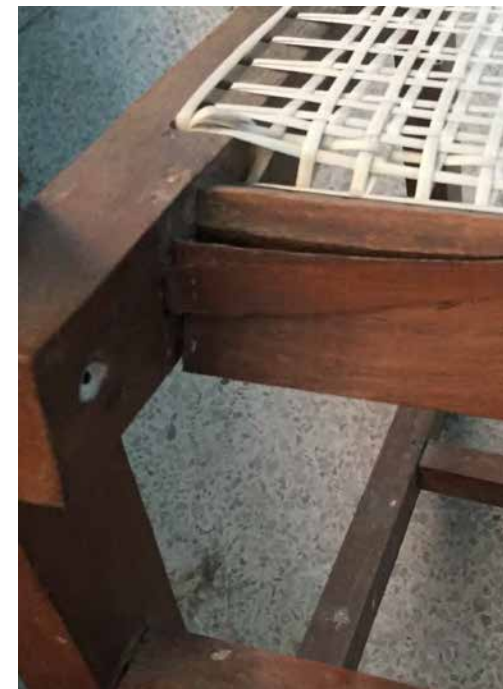
TWISTED MEMBER WITH CRACKS ON REAR SIDE
