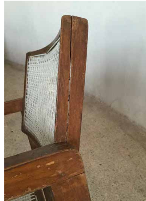
MAJOR CRACK LEFT SIDE OF BACK REST
