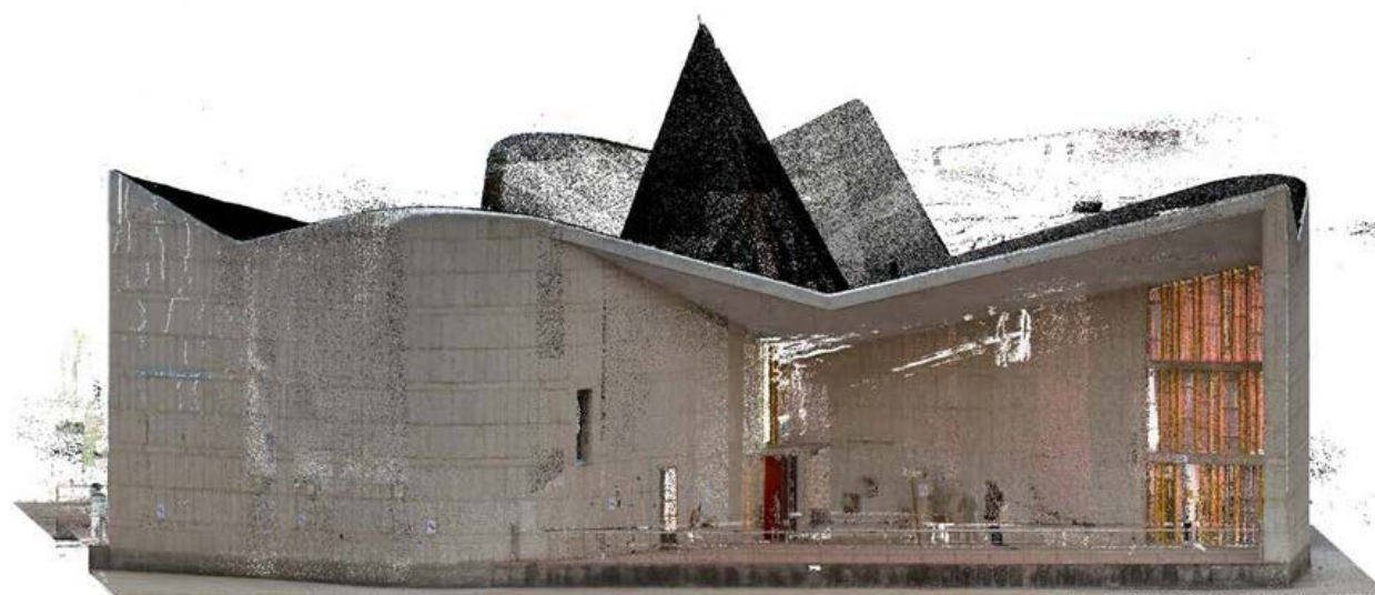
Figure 4. Point cloud prepared by PEGGS for Gandhi Bhawan
