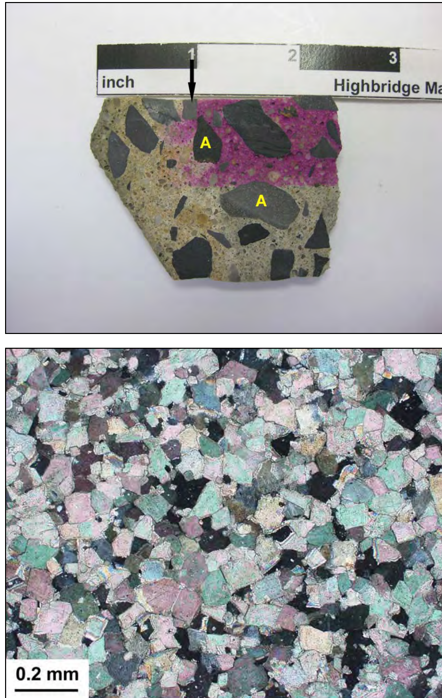
Figure 2: (Upper image) Photograph of the honed cross section of Core #1 with the outer surface oriented toward the left of the image. The crushed stone coarse aggregate (A) can be observed at this scale, though the sample is too small to accurately evaluate the size and distribution. Still, the stone appears to have a nominal top size at the 1/2" sieve. A No. 67 gradation profile is possible. The concentration of aggregate appears normal. A portion of the section is treated with a pH indicator solution. The pink color indicates that a high alkalinity is maintained below about 1" depth. The uncolored upper horizon coincides with the carbonation profile of the concrete. The depth of carbonation is a bit more than desirable at nearly one inch. Any steel reinforcement intersecting this zone could be at risk for depassivation. (Lower image) This XPL photomicrograph illustrates a typical microtexture within the coarse aggregate. The stone is a relatively pure, equigranular dolostone. The angular crystals all consist of dolomite. At this level of purity, the stone is not considered susceptible to alkali-silica reactions. However, dolostone of this character often contains inclusions of reactive chert or chalcedony. None are detected in this particular section.
