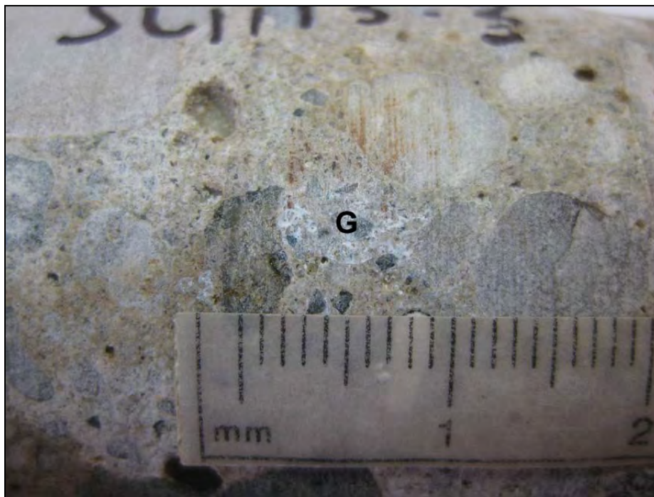
Figure 6: The side of the core sample is shown before further preparation. A few small exudates of gel (G) were observed along the surface when the sample was received. As in Core #2 (Highbridge Report SL1113-02), these exudates show that some unexpanded gel is present in the micropores of the concrete and this likely represents innocuous reactions that have occurred very slowly over the service life of the concrete. No cracking of any kind is associated with these incipient reactions.
