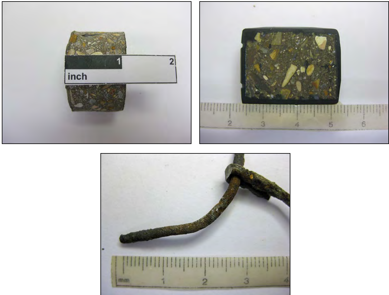
Figure 1: (Upper left) Photograph of Core #1. The sample is shown in side view with its outer surface oriented toward the left. (Upper right) A honed cross section of the dalle de verre is shown. Again, the outer surfaces is oriented toward the left of the image. The numbered units on the scale bar are in centimeters. The binder has a rich brown color typical of aluminite cements with high iron contents. The aggregate is coarse-grained and evenly distributed throughout the thickness. (Lower image) Wire reinforcement is embedded within the core. Note that some moderate corrosion product is evident along the wire. Corrosion of embedded metals could be one possible reason for any cracking noted in the dalle de verre. This is not confirmed in this analysis.
