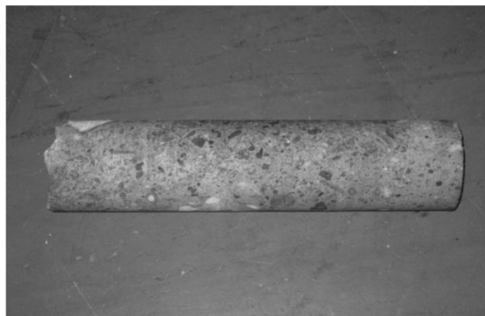
Fig. 3.34. The O-B1 core sample, extracted from pillar B (well-grained aggregate composition visible).
