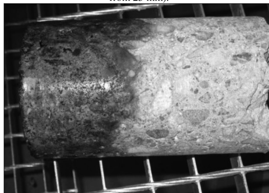
Fig. 3.30. Core sample O-29 – Rainbow test (carbonation depth ranging from 30 mm to 40 mm).
