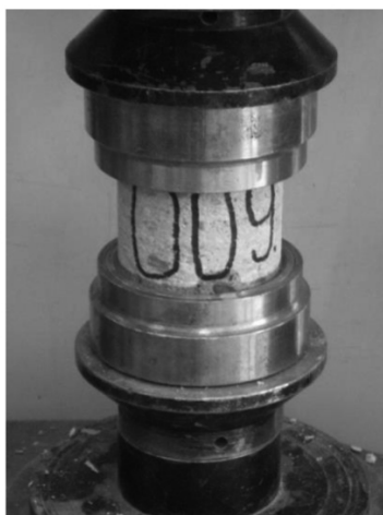
Fig. 3.11. One of specimens adjusted for strength testing with 'capping'.
