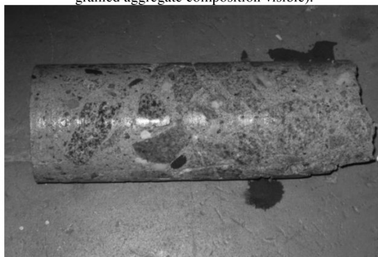
Fig. 3.36. The O-B2 core sample, extracted from pillar B (large granite grains and fine natural aggregate visible).
