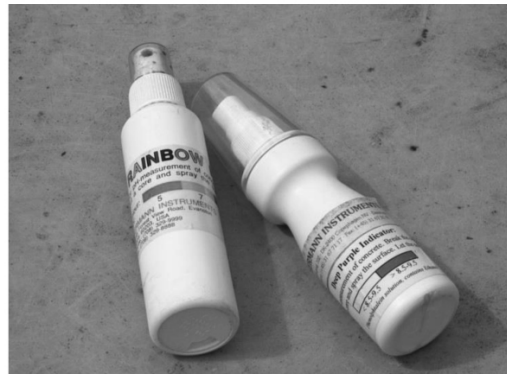
Fig. 3.26. Rainbow and phenolphthalein tests.
