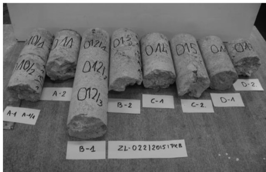
Fig. 3.33. Core samples extracted from supporting pillars.
