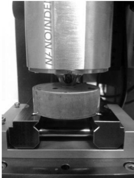
Fig. 3.58. a) The TTX-NHT nano-indentation tester, b) typical indenter curve – loading P in function of displacement h with marked parameters: h_r – remaining indentation, h_i – depth of contact, h_{max} – maximum indentation, S – total stiffness, [78].
