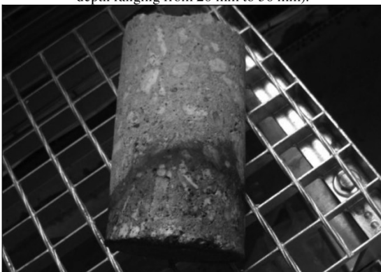
Fig. 3.29. Core sample O-13 – phenolphthalein test (carbonation depth ranging from 45 mm to 55 mm).
