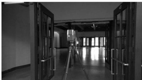
Fig. 4.1. 3D laser scanning device inside the Centennial Hall during measurement.
