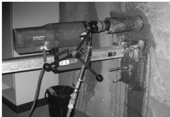
Fig. 3.10. Drilling device used for extracting core samples.
