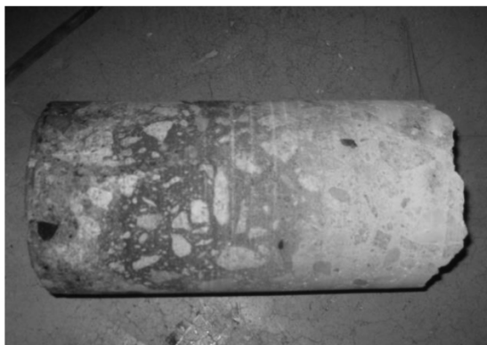
Fig. 3.42. Core sample O-C1 – phenolphthalein test (carbonation depth 35-40 mm).
