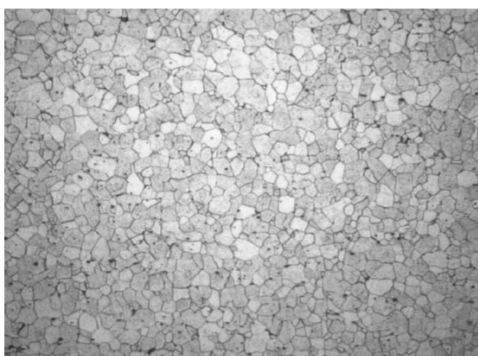
Fig. 3.68. Magnification: approximately 100 X – the microstructure of the second layer of the external belt of the main ring (2) in the middle section. Hardness -109 HV; thickness -13.0 mm.
