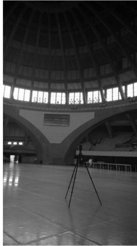
Fig. 4.4. 3D laser scanning device inside the Centennial Hall, under its dome, during measurement
