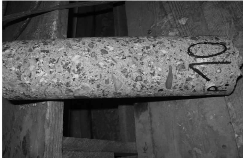
Fig. 3.3. Structure of the analysed concrete as exemplified by a sample from borehole no 10, [8].
