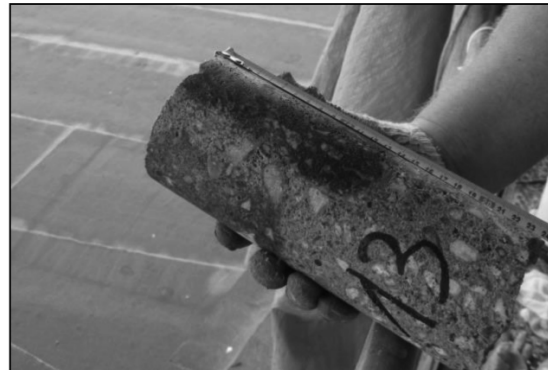
Fig. 3.7. Core sample O-13 – no carbonation (pH ≥ 13), [8].
