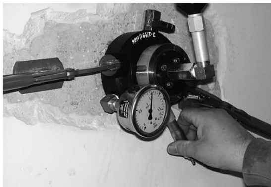
Fig. 3.31. GWT pressure chamber in operation.
