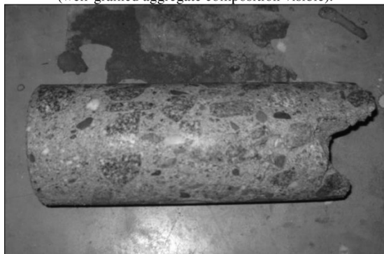
Fig. 3.37. The O-C2 core sample, extracted from pillar C (large granite grains and fine natural aggregate visible).
