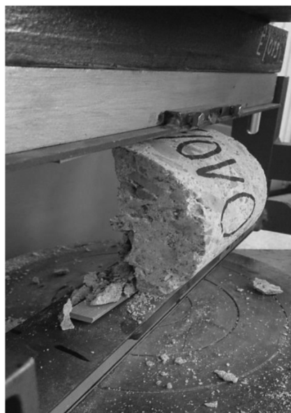
Fig. 3.39. Specimen O-A1/1 after tensile failure.
