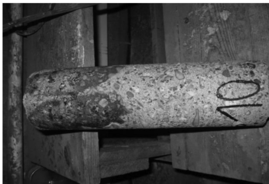
Fig. 3.8. Core sample O-10 – no carbonation ( \text{pH} \geq 13 ), [8].
