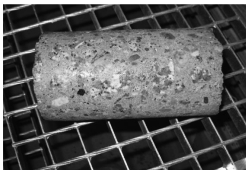
Fig. 3.12. Core sample extracted from the L 17 rib (high content of granite aggregate).
