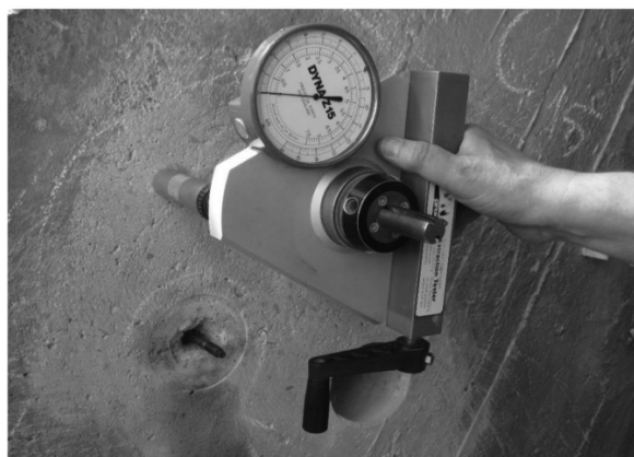
Fig. 3.23. A DYNA device used for tensile strength testing of concrete.
