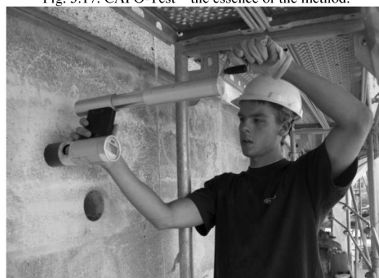
Fig. 3.19. The actuator used in testing.
