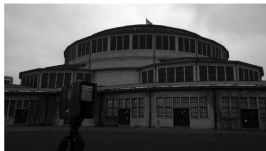
Fig. 4.2. 3D laser scanning device outside the Centennial Hall during measurement.
