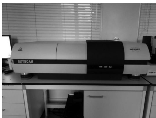
Fig. 3.50. Testing station - SkyScan 1172 micro-CT made by the Bruker company.
