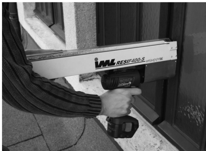
Fig. 3.80. The IML RESI F-400S device used for resistance drilling tests.
