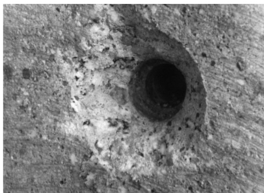
Fig. 3.22. The structure of the tested concrete in the location of one of the Capo-Tests.
