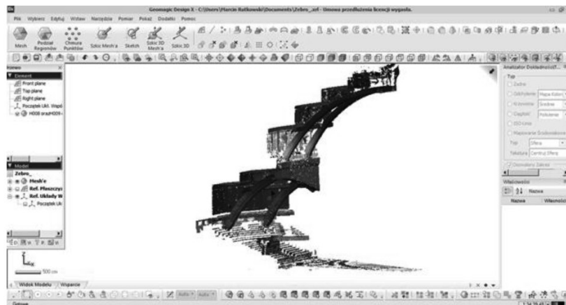
Fig. 4.71. The Geomagic Design X software – a sector of the cloud of points of a rib of the dome and arcades in an isometric view.
