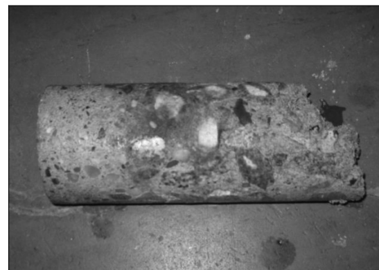
Fig. 3.41. Core sample O-B2 – phenolphthalein test (carbonation depth 70 mm).
