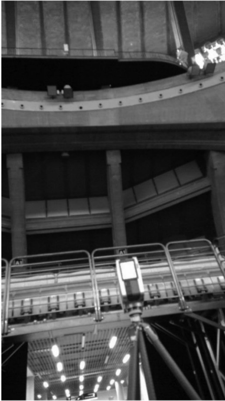
Fig. 4.3. 3D laser scanning device inside the Centennial Hall, under its dome, during measurement
