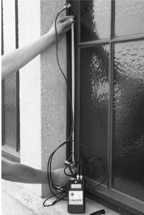
Fig. 3.94. The Fakopp Microsecond Timer device for stress wave testing.
