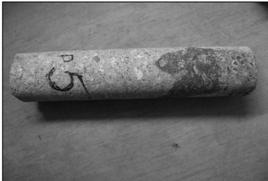
Fig. 3.6. Core sample O-5 – carbonation range - approximately 63 mm, [8].
