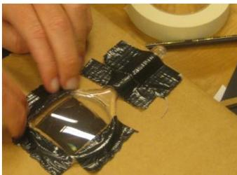
3. Cut out the 1 ½" square with an X-ACTO knife to create an opening. Place a magnifying lens over the opening and tape it to the box, securing the lens on all sides with duct tape.
