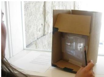
7. Place the framed vellum within the box with the vellum side facing away from the lens. Bring your camera obscura to a window and point the lens out the window. An image will appear on the vellum! Adjust the cardboard frame's position until the image on the vellum is focused.
