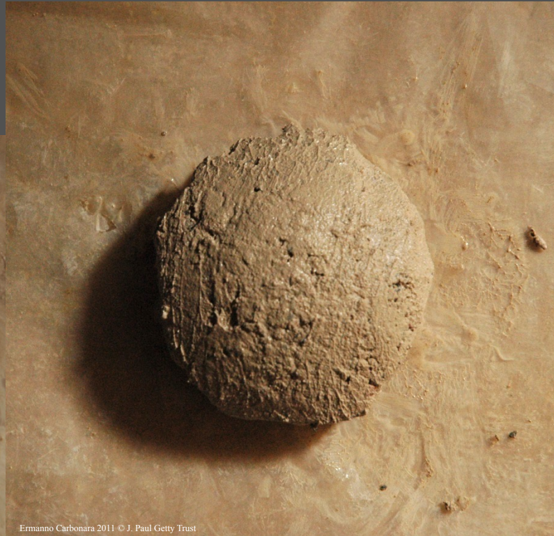
Mortar with the right amount of water
