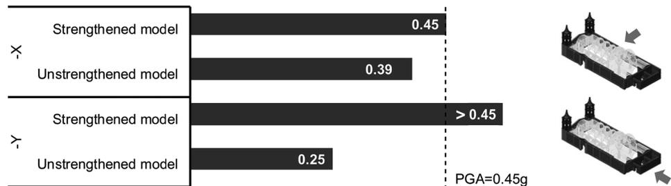
In conclusion, when compared to the unstrengthened model, the results obtained from the pushover analyses on the strengthened model showed an improved global seismic behavior of the structure where higher capacities and ductility were observed.
