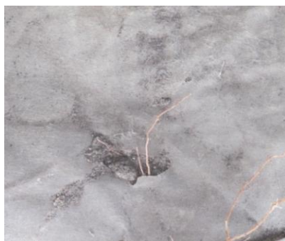
Roots penetrated geotextile in 2 places (left and center); holes may have been created by termites, allowing root access. Small holes created by termites in geotextile (right).
