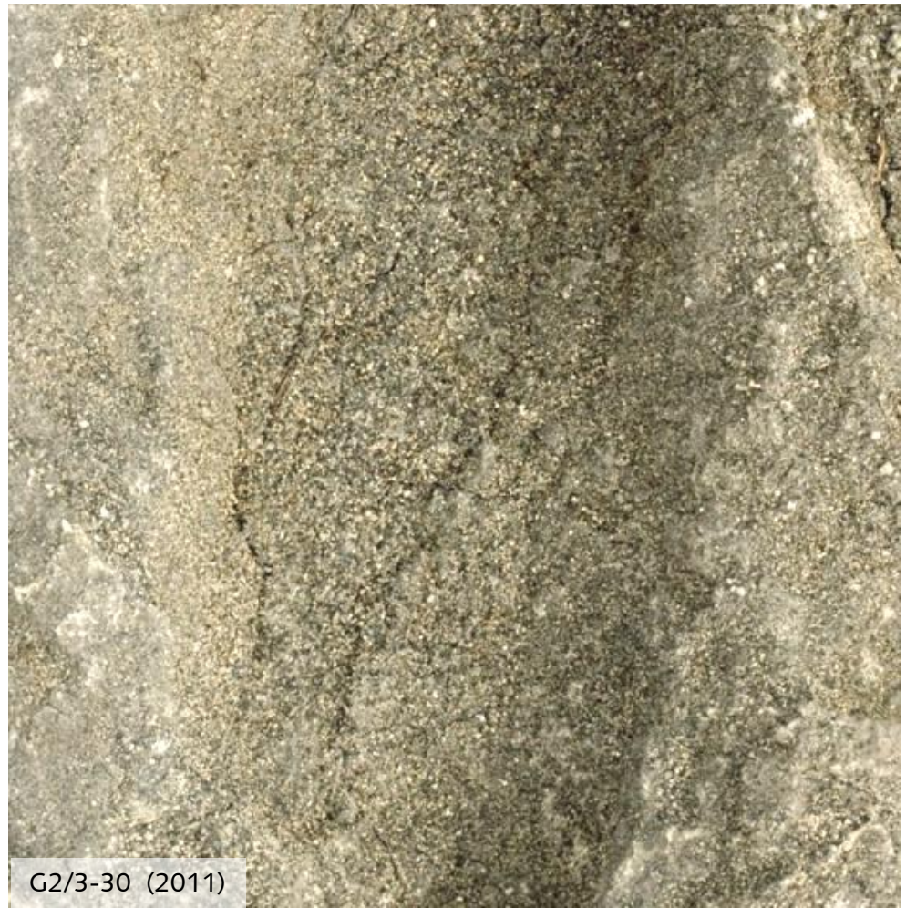
Close-up of G2/3-30 in 1995 and 2011 showing incipient weathering and hairline cracks in 1995 enlarged in 2011
