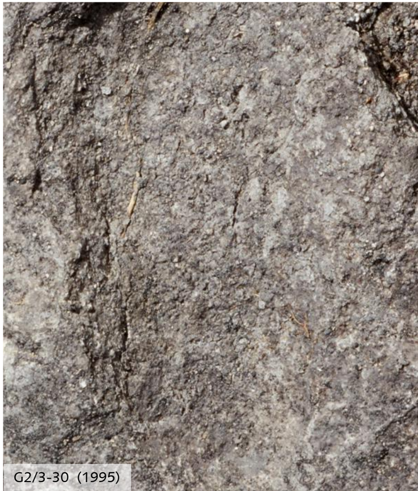
Close-up of G2/3-30 in 1995 and 2011 showing incipient weathering and hairline cracks in 1995 enlarged in 2011
