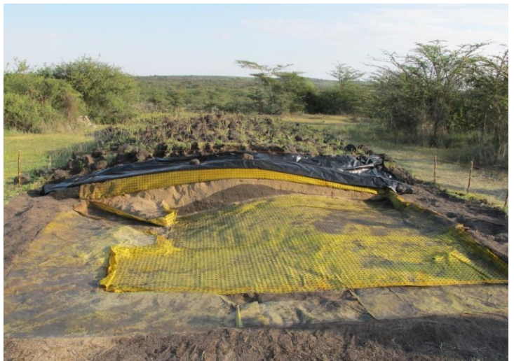
Biobarrier 2 after removal of Layer 3
