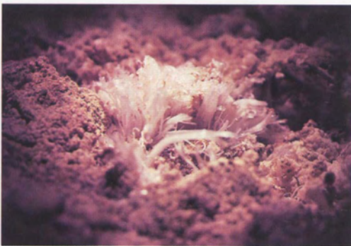
Close-up view showing salt crystals capable of prying the paint layer away from the plaster.
