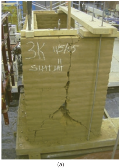
FIGURES 5A AND 5B Specimen 3K after simulation S12 (100% repeated). The in-plane wall and corner connection (a) and the out-of-plane wall (b) are shown.
