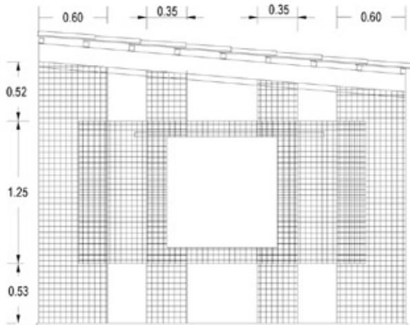
FIGURE 3 Reinforcement distribution for RM-PM75 (dimensions are given in meters).
