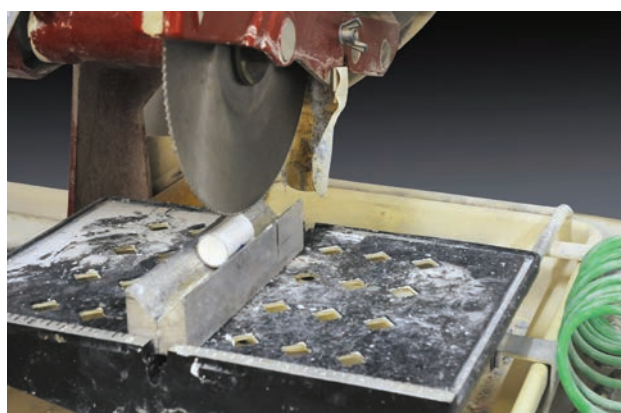
Figure 2.7.5 Slitting of a cylindrical plastic tube with the tile saw. The specimen is held and positioned under the saw by means of a V-shaped holder.
