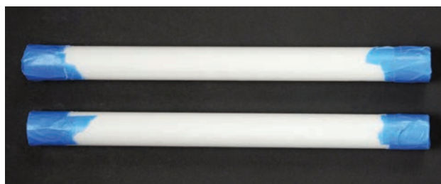
Figure 2.7.4 Columns filled with grout.
