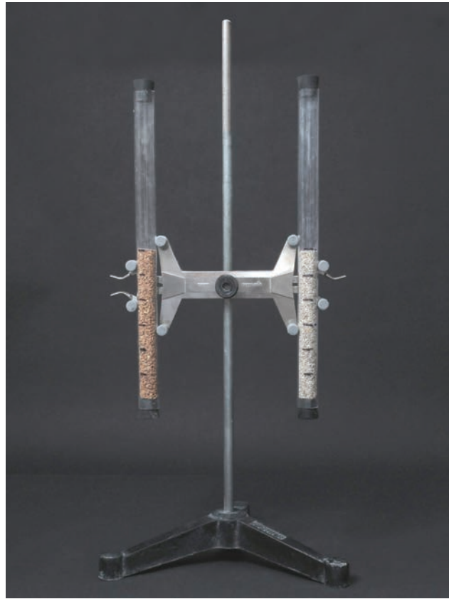
Figure 3.1.1 Columns half filled with crushed brick (left) and crushed travertine (right).
