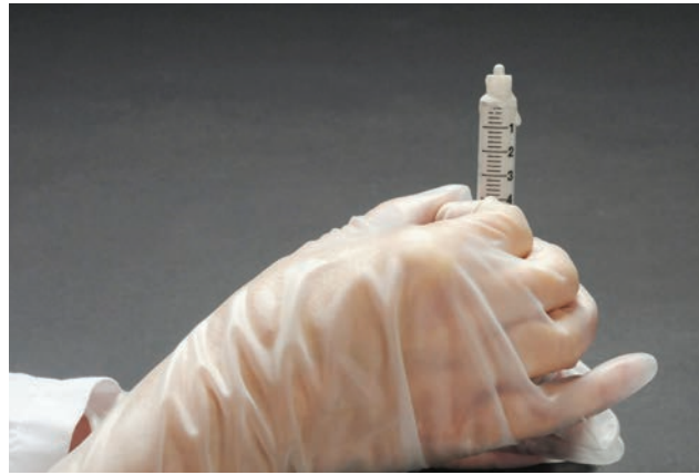
Figure 4.5.1 A syringe filled with grout is tapped to remove air bubbles.
