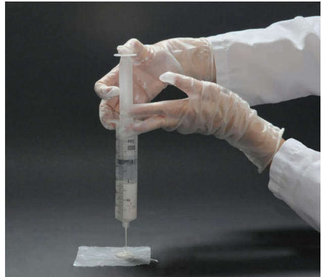
Figure 4.1.4 Applying pressure to the plunger either until grout comes out the tip or until grout stops moving through the granular material.
