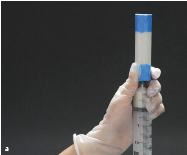
Figures 4.8.2a and 4.8.2b The top of the column sealed with adhesive tape (a), and the column turned upside down (b).
