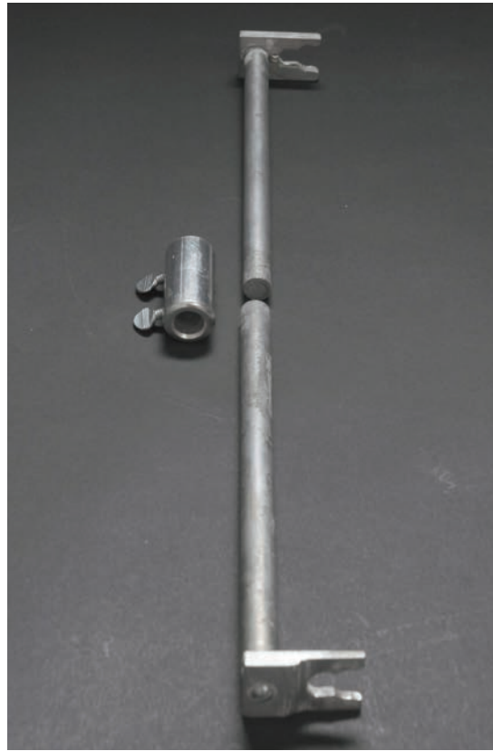
Figure 2.7.3 Example of a metal tie for the injectability apparatus.
