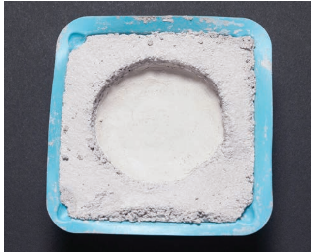
Figure 4.6.6 Specimen exhibiting no drying shrinkage (NS).
