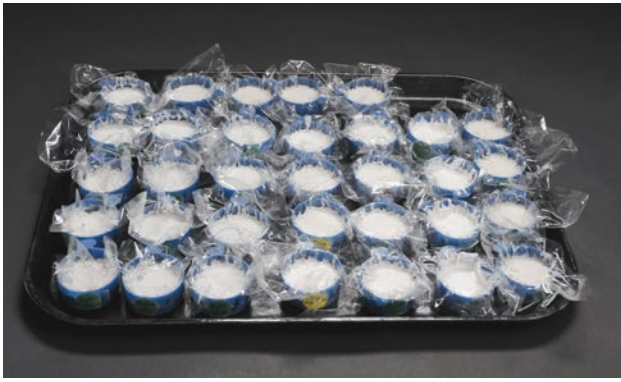
Figure 2.4.3 Shrinkage specimens molded using plastic sheet.
