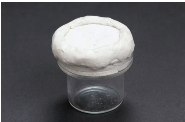
Figure 2.8.4 Prepared dry cup with specimen.
