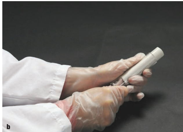
Figures 4.8.3a and 4.8.3b Slitting of a cylindrical plastic tube with a PMMA cutter (a), and removing the cured grout specimen (b).
