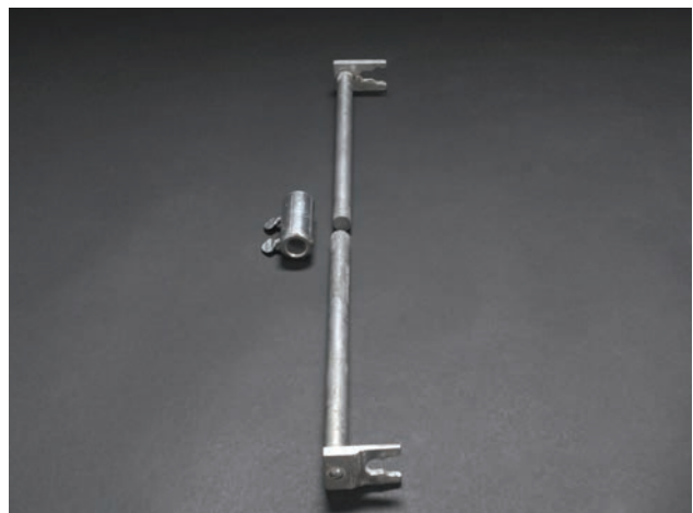
Figure 2.5.3 Example of a metal tie for the injectability apparatus.
