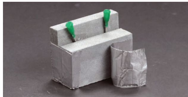
Figure 3.5.2 Preparation of specimen assembly.
