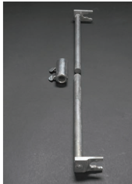
Figure 2.1.5 Example of a metal tie for the injectability apparatus.
