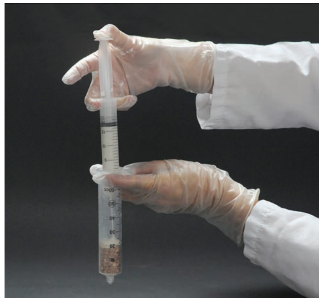
Figure 4.1.2 Injecting 20 mL grout into a 60 mL syringe.
