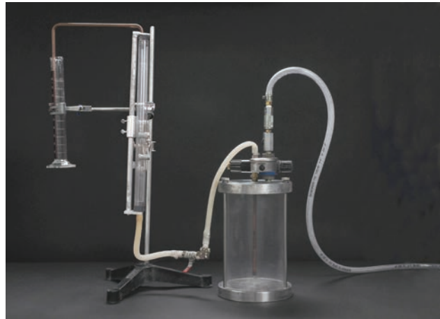
Figure 2.7.1 Example of a commercially available injectability apparatus with an empty column.
