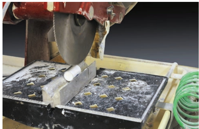
Figure 2.5.5 Slitting of a cylindrical plastic tube with the tile saw. The specimen is held and positioned under the saw by means of a V-shaped holder.
