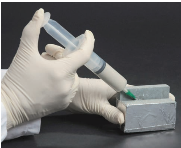
Figure 3.5.3 Injecting grout into the crevice between the stone surfaces.
