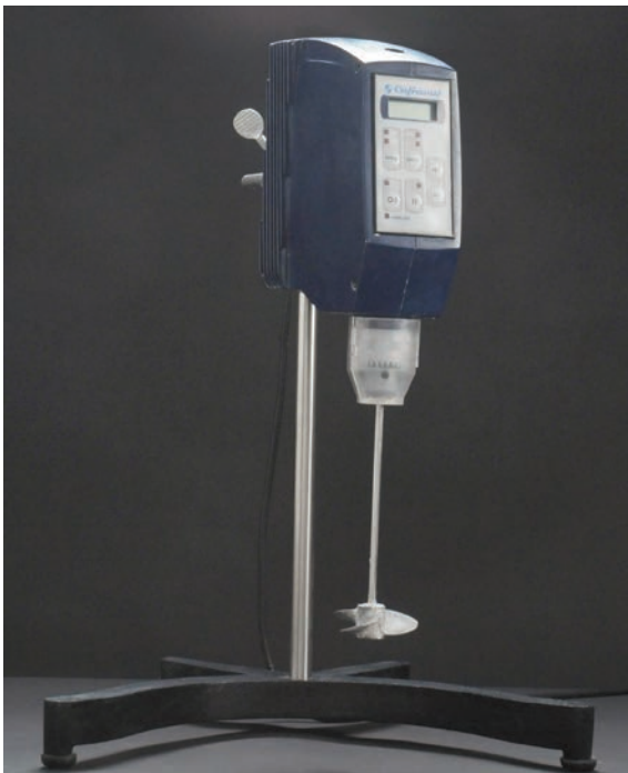
Figure 1.5.1 A universal variable-speed stirrer with three-blade propeller (Caframo Stirrer BDC 3030) for mixing injection grouts.
