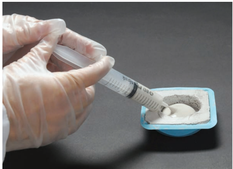
Figure 4.6.5 Grout being injected into a mortar cup.
