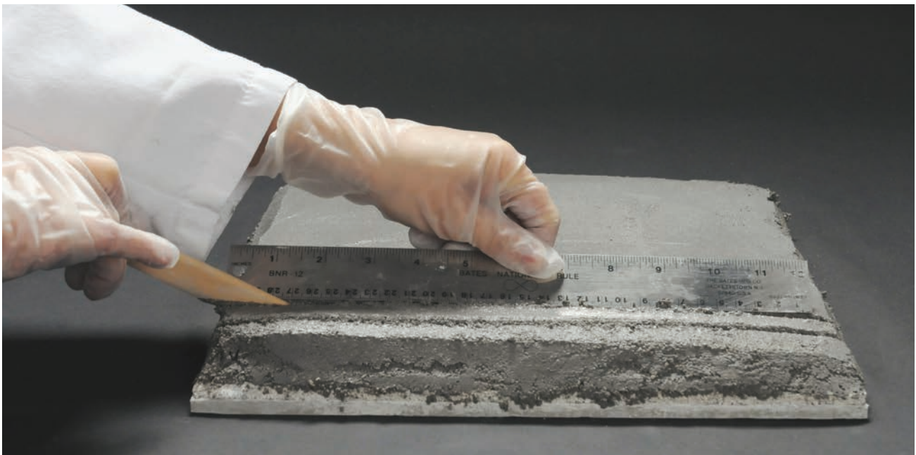
Figure 4.3.1 Making parallel V-shaped channels using a ruler and cutting tool.
