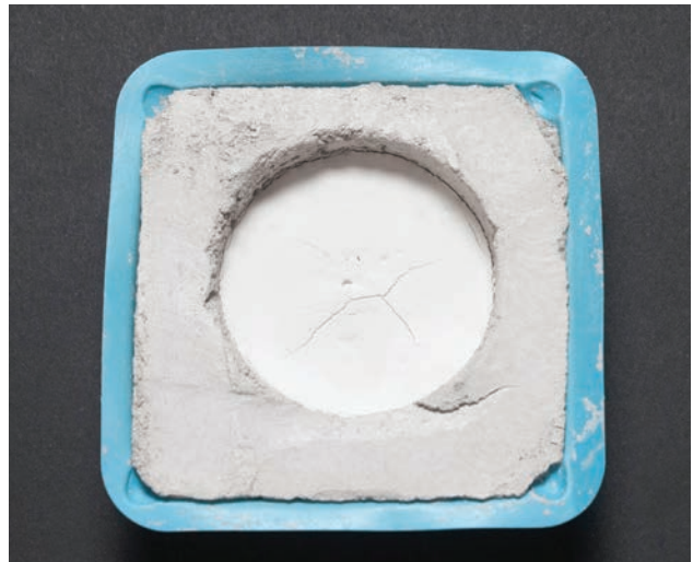
Figure 4.6.7 Specimen exhibiting medium drying shrinkage (MS).
