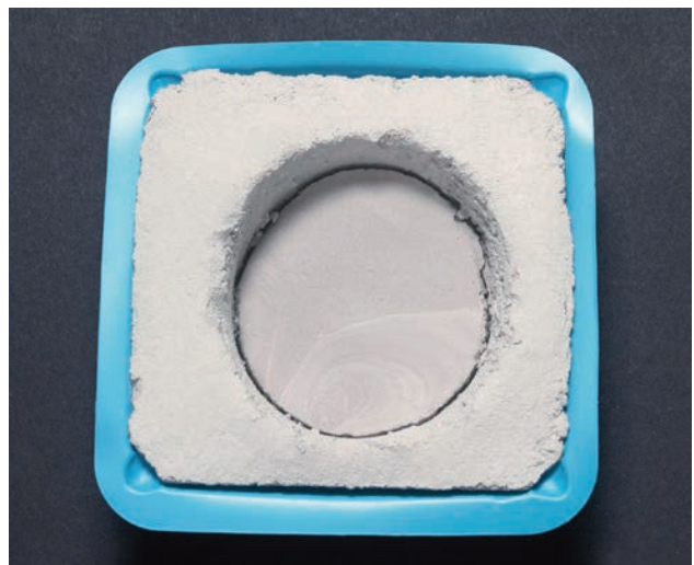
Figure 4.6.8 Specimen exhibiting high drying shrinkage (HS).
