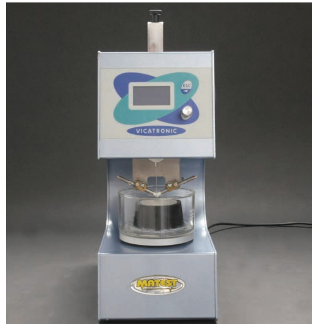
Figure 3.4.1 Automated Vicat apparatus (cement setting tester, appendix B).
