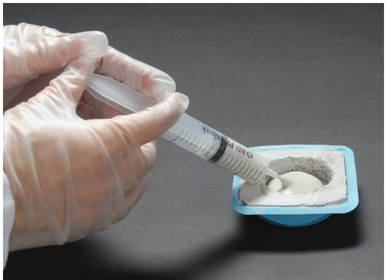
Figure 4.7.5 Grout being injected into a mortar cup.
