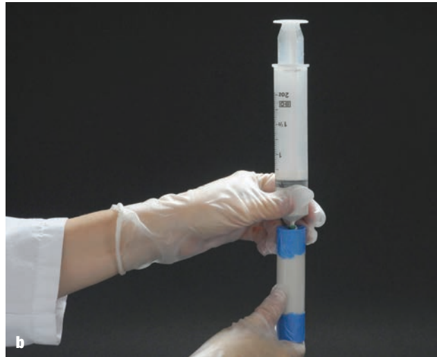
Figures 4.8.2a and 4.8.2b The top of the column sealed with adhesive tape (a), and the column turned upside down (b).
