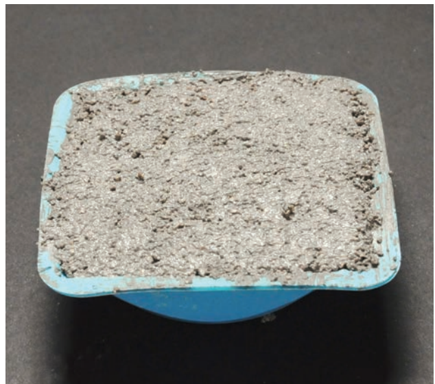
Figure 4.6.1 A weighing boat or shallow container filled with mortar.
