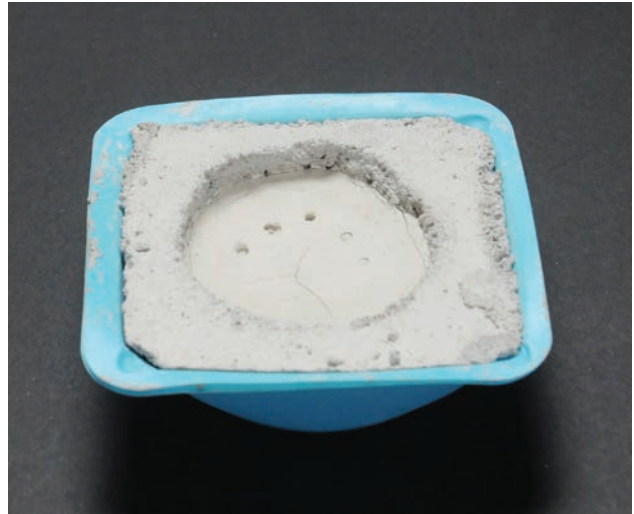
Figure 4.7.7 Final setting, reached after five penetrations.
