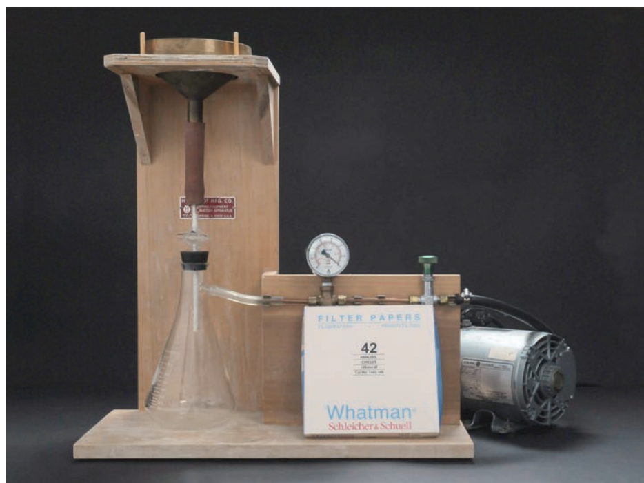
Figure 3.2.1 Example of a commercially available filtration assembly (water retention apparatus, appendix B).
