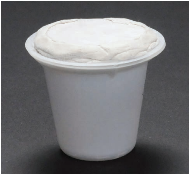
Figure 4.9.2 Cup with cured specimen after sealing.
