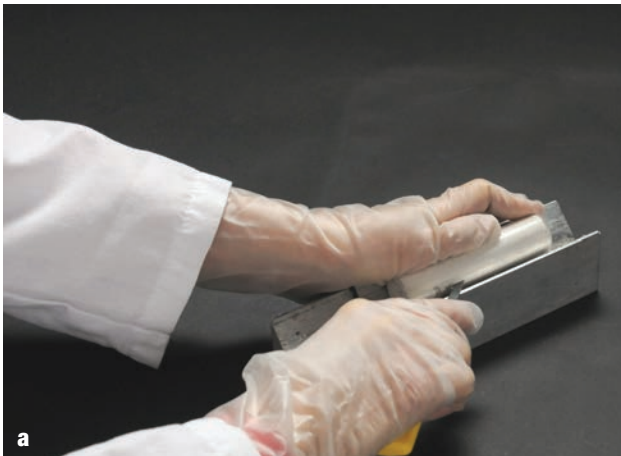
Figures 4.8.3a and 4.8.3b Slitting of a cylindrical plastic tube with a PMMA cutter (a), and removing the cured grout specimen (b).
