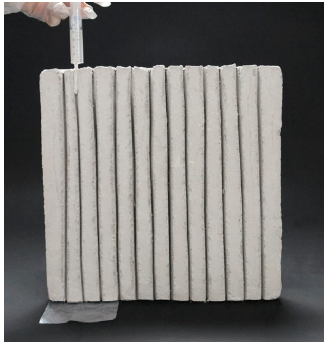
Figure 4.3.3 Injecting 10 mL grout into a channel.
