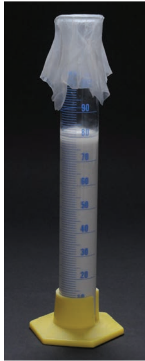
Figure 4.4.1 Grout in a graduated cylinder.
