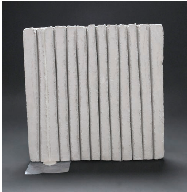
Figure 4.3.4 The distance the grout has flowed is recorded. In this case, grout demonstrated high flow and accumulated at the bottom of the tile.
