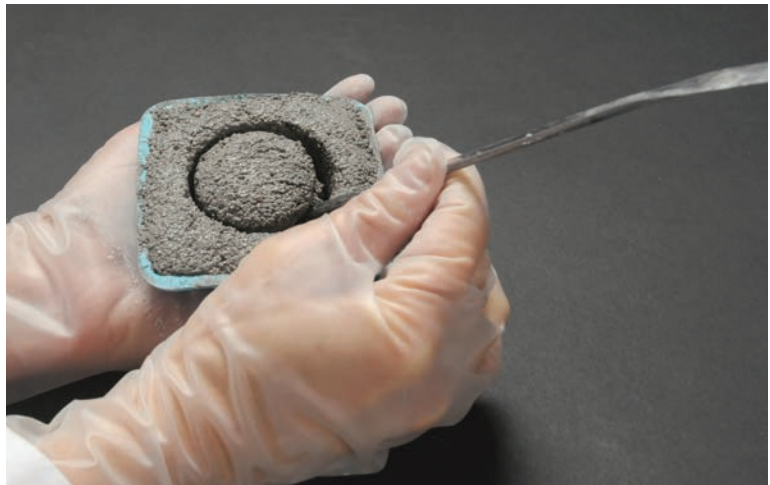
Figure 4.7.3 Removing excess mortar from the cavity.
