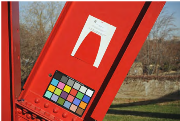
Figure 5 Detail of the paint drawdown in 2006 on Are Years What? (For Marianne Moore) , showing a minimal degree of color shift of the aged paint. Photo by Hirshhorn conservation staff, March 2013. Photo courtesy of the Hirshhorn Museum and Sculpture Garden. © Mark Di Suvero / Spacetime C.C.
