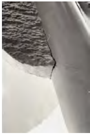
Figure 3 Crack between an aluminum quill and a fiberglass feather observed on one of the Shuttlecocks shortly after their 1994 installation.
