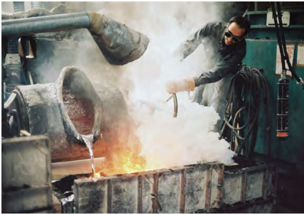
Figure 2 An aluminum alloy casting at the Kunstgiesserei St. Gallen. Photo by Katalin Deér.
