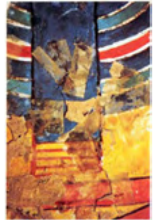
FIGURE 8, TOP LEFT. SALT EFFLORESCENCE ON THE PAINTED SURFACE.
