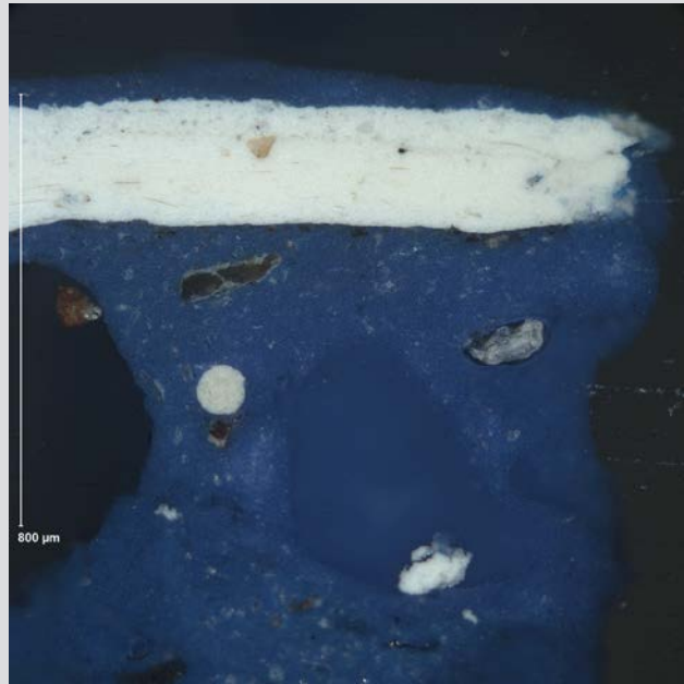
FIGURE 1.32A Cross section West Exterior_13. Crossed polarizing filters. 10× objective.
