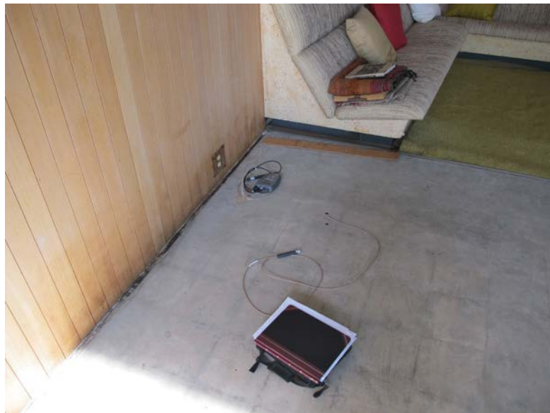
FIGURE 4.24 Data logger with temperature and humidity sensor in the concrete floor slab, 2011. Photo: Shin Maekawa
