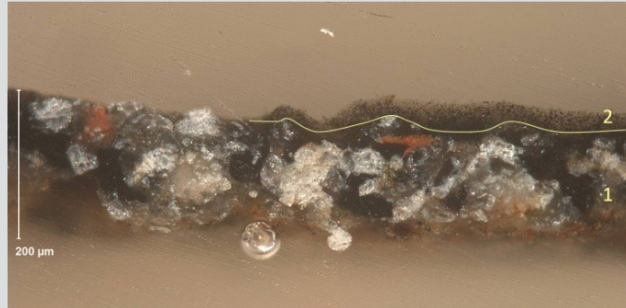
FIGURE 1.28A Cross section South Exterior_11 Fragment B. Crossed polarizing filters. 10x objective + 1.5x magnifier (= 15x).
