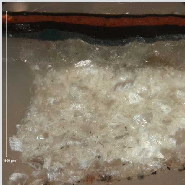
FIGURE 1.37A Cross section Eames House_putty#1b-2; partially uncrossed polarizing filters. 10x objective.
