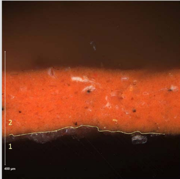
FIGURE 1.15A Cross section East Exterior_4. Crossed polarizing filters. 20× objective. Annotated to show layer structure.
