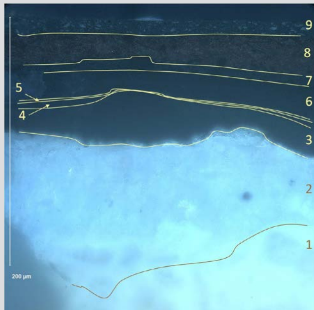
FIGURE 1.37C Cross section Eames House_putty#1b-2; UV fluorescence. 50x objective.
