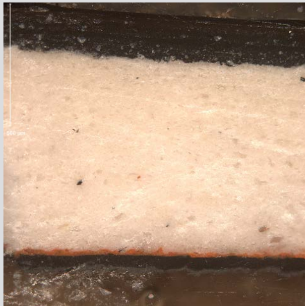
FIGURE A1.4A Cross section of sample Eames House_putty#1a; visible light.
