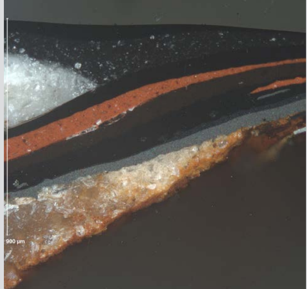
FIGURE 1.22B Cross section North Exterior_10. Crossed polarizing filters. 10x objective.
