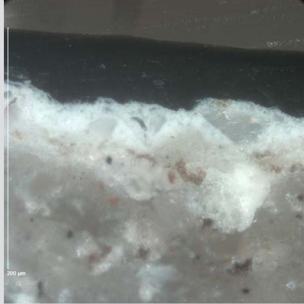
FIGURE 1.33A Cross section West Exterior_14; Crossed polarizing filters. 50× objective.
