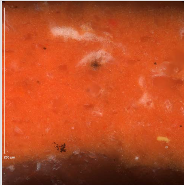
FIGURE 1.15E Cross section East Exterior_4. Crossed polarizing filters. 50x objective.
