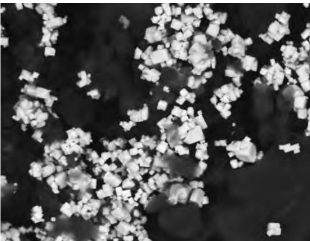
FIGURE 9 Well-formed cubic crystals of sodium chloride below the paint layer (also at the clay-conglomerate interface).
