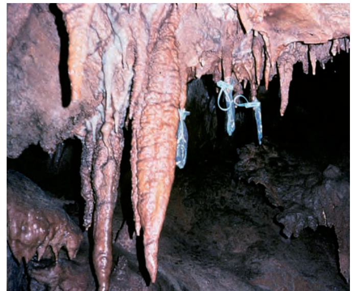
FIGURE 4 Rubber condoms are attached to some cave formations to measure the quantity of water entering the cave system. These data may be correlated with both external data (e.g., rainfall) and internal cave data (e.g., visitation numbers and frequency, desiccation). Courtesy of Jenolan Caves Reserve Trust
