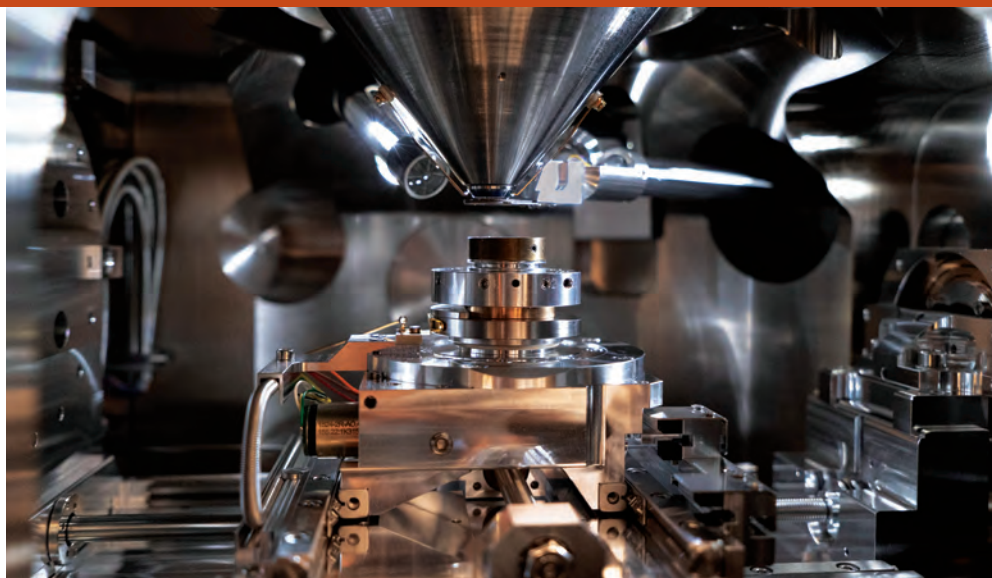
Inside the sample chamber of a variable pressure scanning electron microscope. Photo: Andrzej Liguz, for the GCI.
