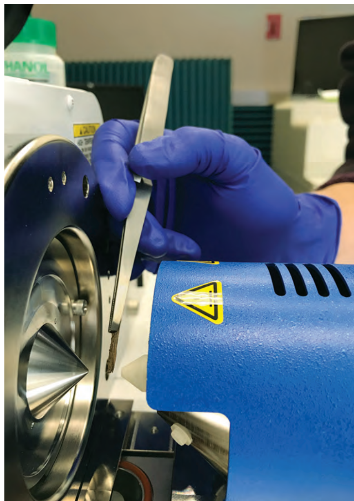
Analysis of a wood sliver using DART (Direct Analysis in Real Time). Traditional methods for analysis of wood phytochemicals require large samples, tedious solvent extraction protocols, and long analysis times using GC-MS or LC-MS. DART overcomes these problems through its unique design and is being applied in wood species identification. Photo: courtesy of the National Fish and Wildlife Forensic Laboratory.
