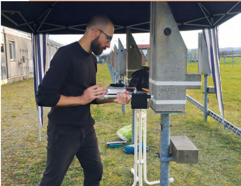
Davide Gulotta of the GCI testing a field-portable air permeametry device at Holzkirchen, Germany, where sandstone samples were exposed to the environment as part of a German government-funded project to understand the deterioration and conservation of historic building materials. Photo: courtesy of Katrin Wilhelm, University of Oxford.
