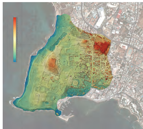
Digital surface model of the Paphos site showing elevation of topographical and archaeological features, with red indicating the highest level and blue indicating the lowest. Image: Carleton Immersive Media Studio, for the GCI.
