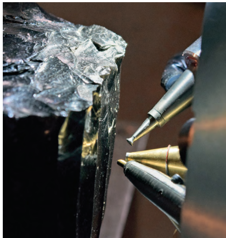
Ion beam analysis of an obsidian core for blade production from the Final Neolithic dwelling site of Sa Duchessa (Cagliari, Sardinia, Italy), dating from the beginning of the 4th millennium BCE. Photo: © C. Lugliè. C2RMF / Vanessa Fournier. Appeared in "FIXLAB Transnational Access: The Opportunity for Cultural Heritage Scientists to Access Large Scale Facilities," by Claire Pacheco, published in Techné .
