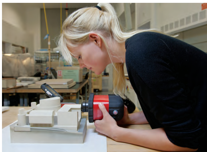
In the conservation studio at the Getty Research Institute, Julia Langenbacher of the GCI conducts FTIR analysis of an architectural model of a proposal for Disney Hall by architect James Stirling. Analysis using portable FTIR instruments can be carried out without the need for sampling, greatly expanding the range of objects that can be studied. Photo: Scott S. Warren, for the GCI. With permission of the Canadian Centre for Architecture, Montreal.
