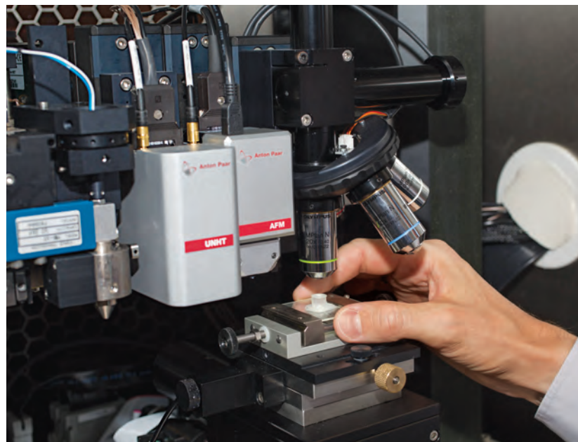
From left to right: microindenter/scratcher; ultra nanoindenter; atomic force microscope; and optical microscope, inside a climatic chamber. A cross-sectional sample is under the optical microscope. Photo: Evan Guston, for the GCI.
