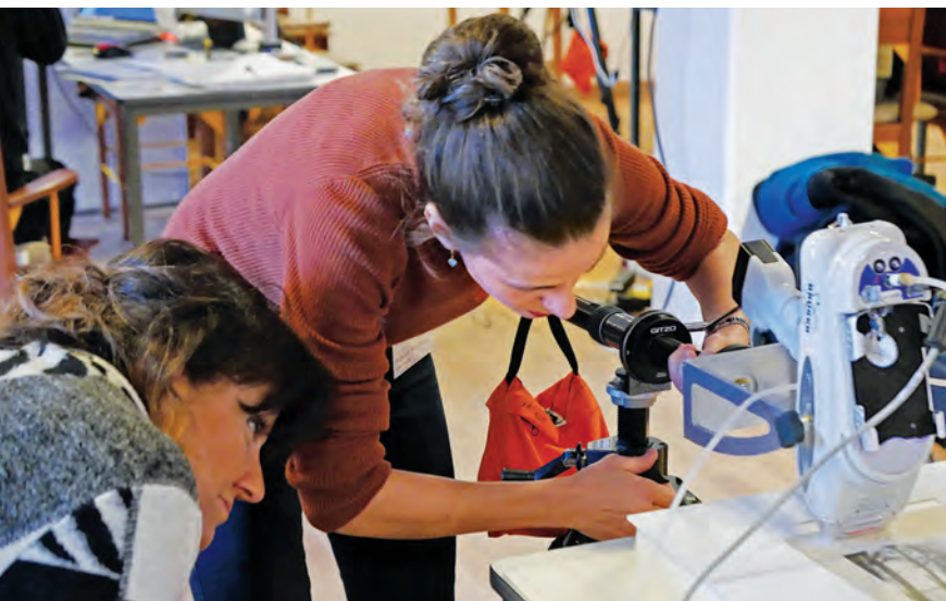
Participants adjust a portable XRF unit before taking a measurement during the GCI's XRF Boot Camp workshop held at the Bonnefontenmuseum, the Netherlands, in 2016. Photo: Stéphanie Auffret, GCI.
