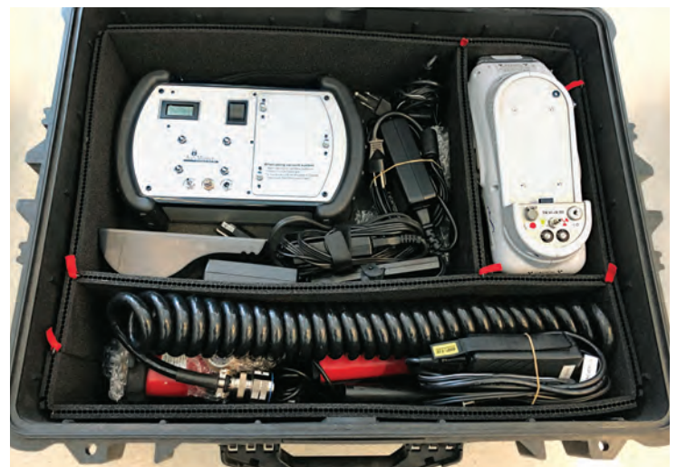
Three handheld instruments—XRF, FTIR, and a digital microscope —packed into a 24 × 20 × 12 inch (approx. 60 × 50 × 30 cm) protective transport case prior to travel, allowing elemental, molecular, and visual data to be collected in situ. Photo: Art Kaplan, GCI.
