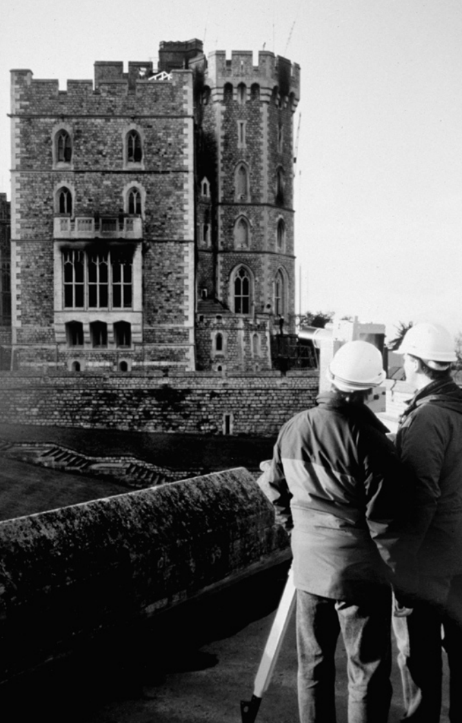
English Heritage staff conducting a photogrammetric survey of the exterior of Windsor Castle. Documentation can provide a lasting record of cultural heritage—essential for conservation or recovery from an unforeseen catastrophic loss. When a disastrous fire in 1992 destroyed much of Windsor's St. George's Hall and Grand Reception Room, English Heritage was able to use photographic documentation taken years earlier, as well as new material, to guide restoration work. Photo: Courtesy of English Heritage, with acknowledgment of the Royal Household at Windsor Castle.
