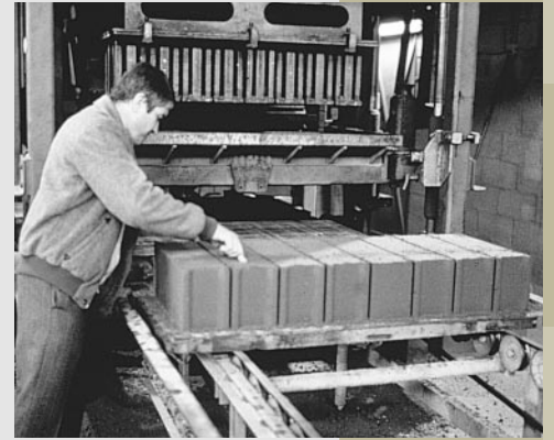
Right, bottom: Mechanized production line of stabilized compressed earth blocks in Isère, France. Photo: H. Guillaud (© CRATerre-EAG).
