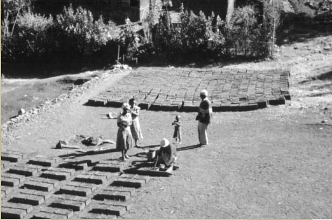
Right, top: Mud brick production for use in the construction of homes in Yunnan Province, China. Photo: Neville Agnew.
