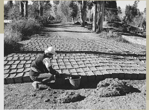
Right, top: Mud brick production for use in the construction of homes in Yunnan Province, China. Photo: Neville Agnew.
