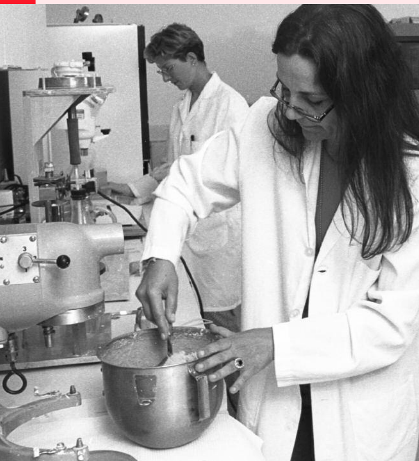
Conservation guest scholar Maria Isabel Kanan preparing a lime mortar in the GCI's accelerated aging lab. The Institute's Conservation Guest Scholar program provides opportunities for conservation professionals to pursue interdisciplinary scholarly research among the GCI's staff and laboratories. Photo: Dennis Keeley.
