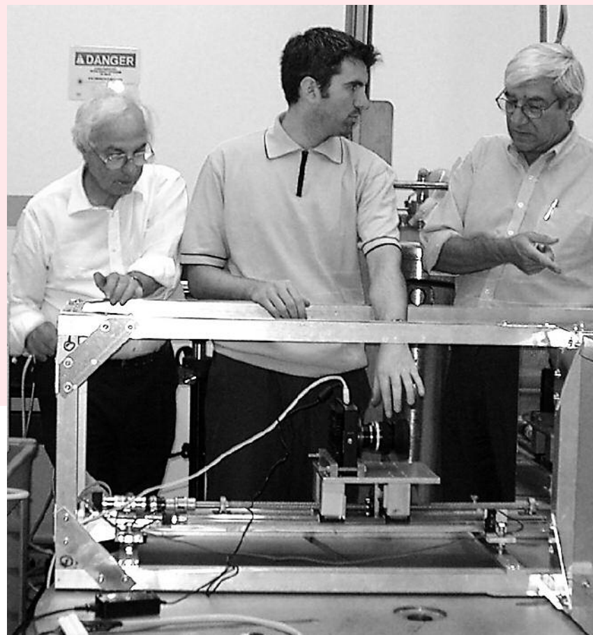
Franco Casali and Alessandro Pasini of the University of Bologna and Giacomo Chiari of the GCI discussing the assembly of an X-ray tomography system in the GCI's Museum Research Lab. The GCI has formed a partnership with University of Bologna experts to develop a X-radiography system capable of performing CT scans on large bronze objects. Photo: Gary Mattison.
