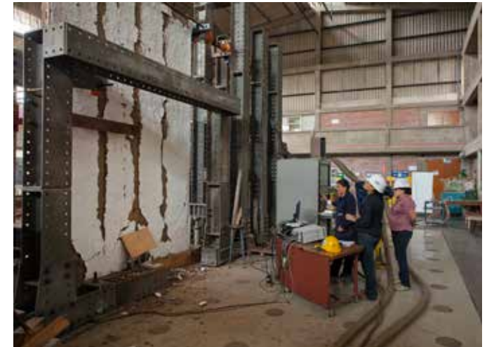
Above: Shear strength tests via lateral displacement of mock up of a quinchá panels, a vernacular building technique, at the Pontificia Universidad Católica del Perú. Photo: Scott S. Warren
