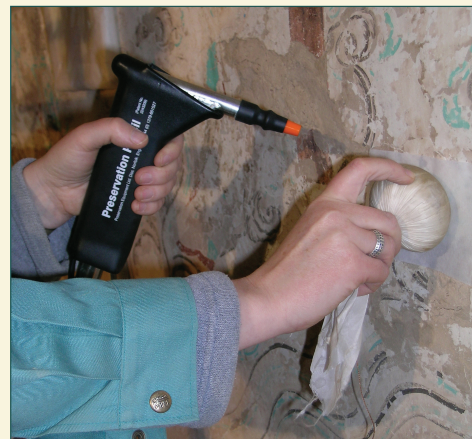
鉴于泥质地仗的脆弱状况和壁画对水的高度敏感，降低可溶盐只能限于局部选定的区域。使用超声波加湿器配合吸水棉纸可以用来吸收表面及表面下的盐分。 Reduction of soluble salts was limited to select areas given the fragile condition of the earthen plaster and the water sensitive painting. An ultrasonic humidifier was used with absorbent tissue to absorb surface and subsurface salts.
