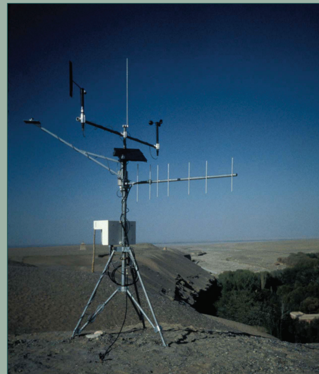
莫高窟崖顶设置有全自动气象站可监测降雨强度与雨量、空气温度、相对湿度、风速和风向等气象因子。 A weather station at the top of the cliff measures rainfall intensity and amount, air temperature, relative humidity, and wind speed and direction.
