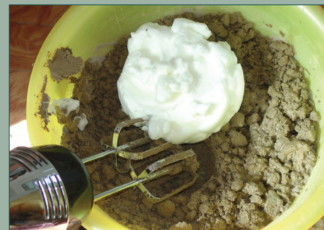
第85窟筛选出来的灌浆材料包括本地清洗过的粘土、玻璃微珠(Scotchlite K1®)、碾碎过的浮石、搅拌好的蛋清和蒸馏水。 The adhesive grout formulated for Cave 85 included local washed clay, glass microspheres (Scotchlite K1®), crushed pumice, whipped egg white and distilled water.
