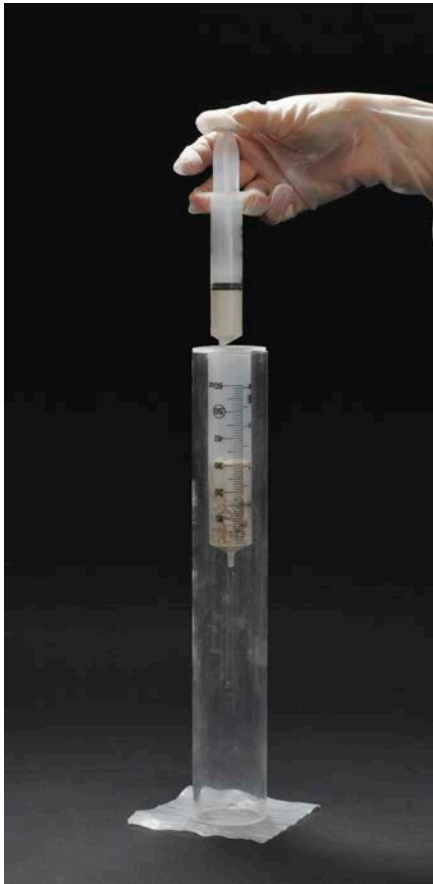
Figure 4 Flow with syringe test of Bresciani Malta 6002 into dry crushed travertine, classified as difficult
