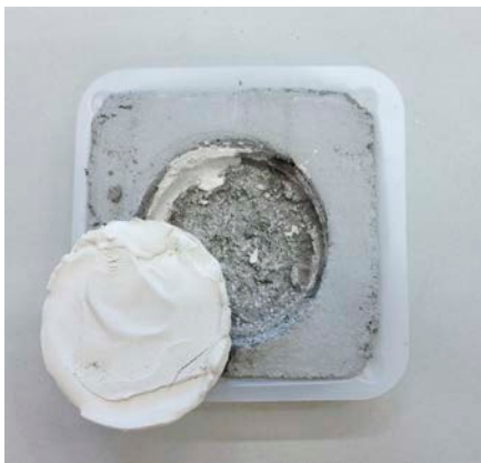
Figure 7 Drying shrinkage test. ICCROM (left), ICCROM_w and ICCROM_w_NHL 2 (right) filled mortar cups
