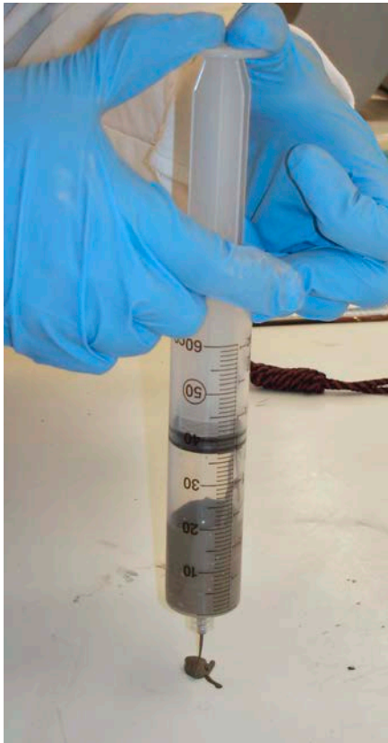
Figure 2 Syringes filled with crushed travertine
