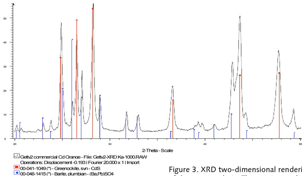
Figure 3. XRD two-dimensional rendering of the same analysis. The continuous lines are identified as cadmium sulfite and selenite (CdS /CdSe – in red), while the dotted lines are due to barite (barium sulfate – in blue), added as a filler.
