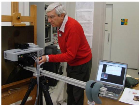
Figure 7. The distance between the instrument and the object must be exactly 2 mm. This is achieved using a fine tuned stage. The red laser line seen in the small window of the PC allows for positioning as precise as 20  $\mu\text{m}$  in the focal plane. Photo: C. Namowicz.
