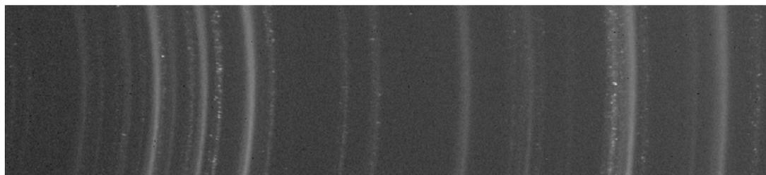
Figure 2. Image of the CCD detector. One can see the continuous diffraction lines, indicating that the crystals are very fine as randomly oriented. There are a few dotted lines, due to the presence of large crystals in a poorly crushed powder. The sample analyzed was a cadmium orange commercially manufactured color.
