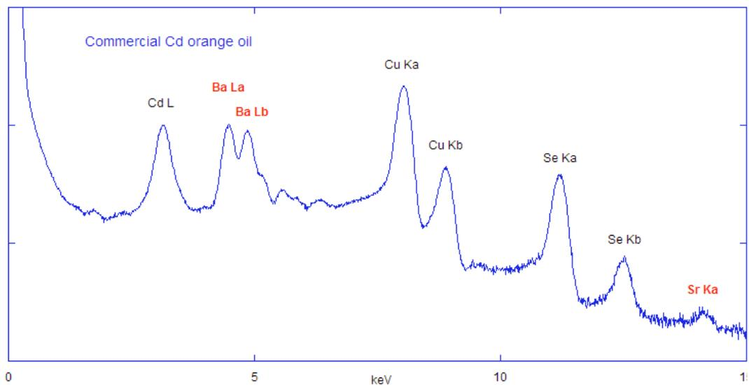
Figure 4. XRF pattern which shows cadmium, selenium and, unexpectedly, barium. The two lines of CuK $\alpha$  and CuK $\beta$  are due to the X-ray tube emission and are always present.
