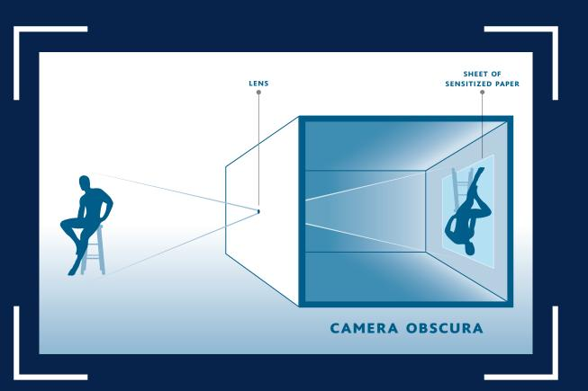
invention of photography. The camera obscura relies on the essential components required to make a photograph—a dark chamber fitted with a lens, sensitized paper, and light. After
